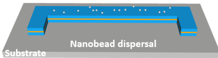
Figure 6.4. Schematic presentation of the nanobead process Step-I i.e., nanobead dispersal. The dark gray colored area represents the substrate ( \text{Si}|\text{SiO}_x ), while the layers with sky-blue color represent the FM electrodes (top and bottom). The sandwiched dark yellow colored layer represents the organic molecular layer (or the spacer layer). The white spherical-shaped objects on the top surface (capping layer) of the hybrid trilayer stacks are the silica nanobeads, that will be used as a shadow mask to define the cross-section of the vertical nanopillars during the \text{Ar}^+ -ion etching step (Step-II).[33]
