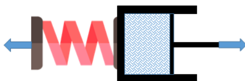
Figure 1.5: The schematic representation of a serial connection of a Hookean spring and a Newtonian dashpot.
