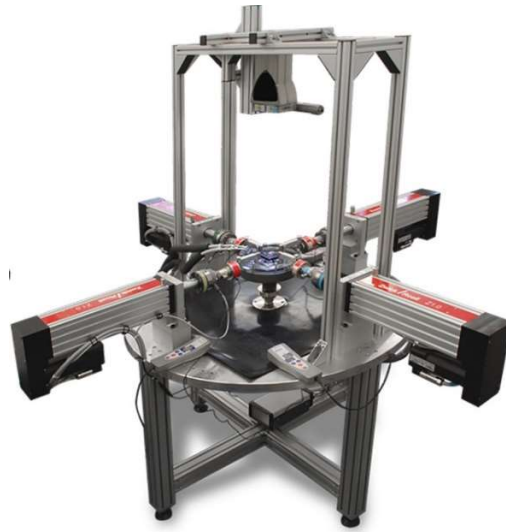
Figure 81. Zwick biaxial tensile test machine (Zwick, 2018)
