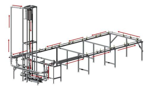
Fig. 2.5 Fluid circuit in the hydraulic loop.
