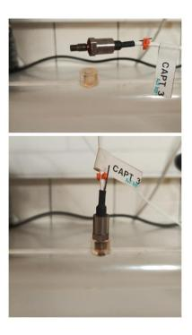
Fig. 2.11 Pressure sensors.
