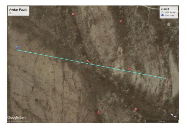
Figure 2.26 Location map of ground penetrating radar profiles in Z1 zone. The zone location is in Figure 2.23. Light blue lines indicate the profiles at the RTA50 MHz, 500 MHz, and 250 MHz antenna. The blue symbols are indicating the start points and name of profiles. The red symbols are representing fault trace.
