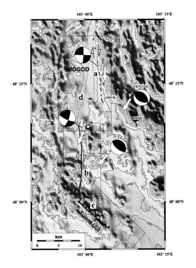
Figure 2.5 Summary map of the 1967 Mogod earthquakes (see Figure 2.4 for location). The main surface fault ruptures (b and c) are shown as heavy lines and are taken from (Baljinnyam, et al., 1993). The three main shock sub events (marked 1, 2 and 3) and the mechanism of the principal aftershock (670120) are taken from our analysis of the P and S waveforms. Slip vectors are shown as large white arrows, after (Bayasgalan & Jackson, 1999b).
