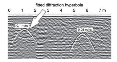
Figure 1.16 Radar velocity analysis by diffraction hyperbola fitting. After (Cassidy N., 2009).
