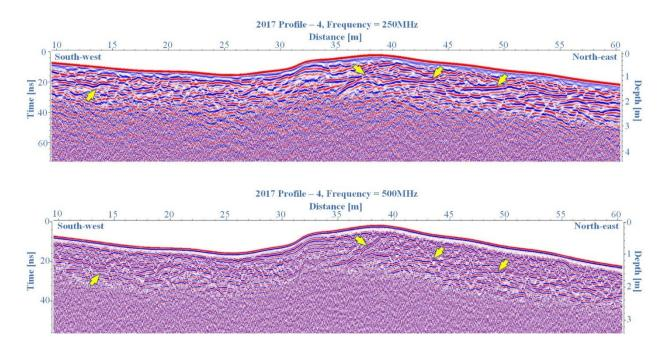
Figure 2.9 GPR result image of the Profile-4 (acquired the June 2017) interpretation of the zone 2 (back-thrust structured) of the Mogod active fault (Figure 2.6c). First figure is 250MHz antenna result image, yellow arrows show the reflections from layers. Second figure is 500 MHz antenna result image, orange line is strong reflected layers.
