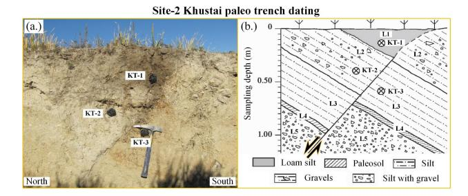
Figure 4.8 OSL dating result of east wall of the trench, excavated in 2011, sampled in 2011, Khustai active fault. a.) photo of sampling strategy from east wall of Khustai trenching site, b.) interpreted image of sampling strategy for the dating and fault movement.
