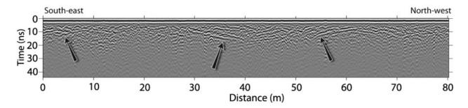
Figure 2.34. Example of a 500 MHz profile crossing paleo-channels and recorded in 2010 to verify the presence of the paleo-channel in the GPR data before the precise work on "cubes". Its location is displayed in Figure 2.33 (blue line). Black arrows highlight dipping reflections, which are related to the flanks of the channels, after (Dujardin J.-R., 2014).
