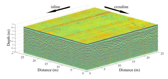
Figure 2.38 Pseudo-3D data cube of the C1 cube obtained with 500 MHz shielded antenna in the paleo river channel of the Emeelt active fault. Inline arrow pointed measurements direction of the GPR profiles parallel to the T3 and T4 trenches (see Figure 2.33 for the locations). Crossline arrow pointed measurement direction of the GPR crossed profiles.
