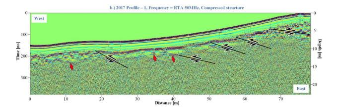
Figure 3.22 The result of GPR image of the profile P1 of PPr8 zone (acquired in August 2017) obtained with RTA 50 MHz antenna in the Songino fault study area S2 (see Figure 3.21). The red arrows indicate underground high reflected GPR anomalies, the black arrows show the movement direction.
