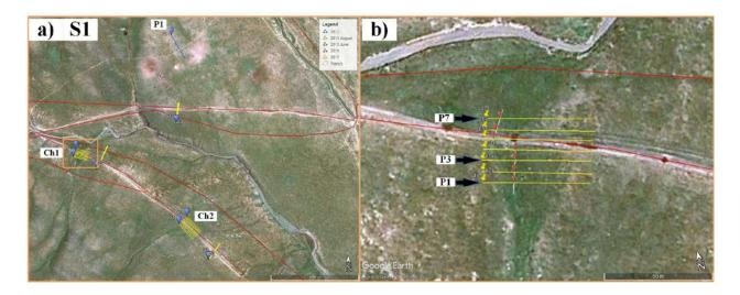
Figure 3.19 Location Map of the GPR profiles acquired in August 2017, S1 zone. a) The GPR survey zone S1as shown in Figure 3.2. b) A magnified map of the profile area (orange square), yellow lines indicate the GPR profiles crossing the paleo river channel. The red lines show the fault traces, the yellow symbols indicate the initial position of the measurements, red symbols (F) indicate the intersection of the fault traces on the surface rupture with the profile.
