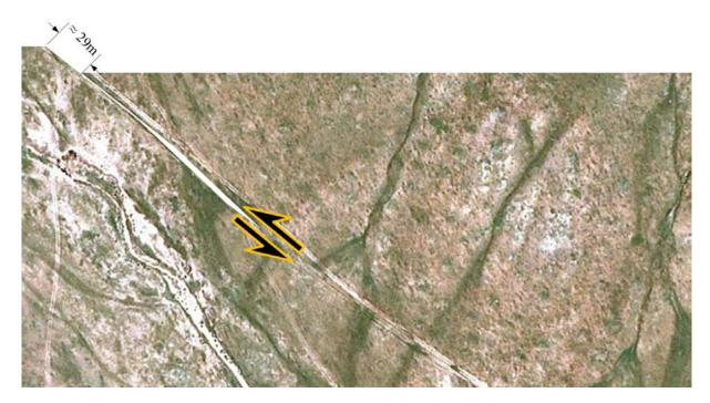
*Figure 4.13 Reconstruction of the paleo-river channel movement on the left lateral strike-slip zone. Cumulative left lateral strike slip offset is approximately 29meter. Google Earth 2009.*
