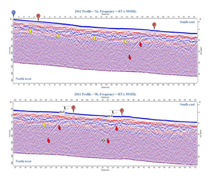
Figure 2.29 Result of GPR image of the profile P9 (acquired the October 2011) obtained with RTA 50 MHz antenna in the Avdar fault. The GPR image shows a clear fault structure (red arrows), and surface rupture location is red colored symbols (F), two dipping angles approximately of 18.4°, yellow arrows are pointing bed rock layer.
