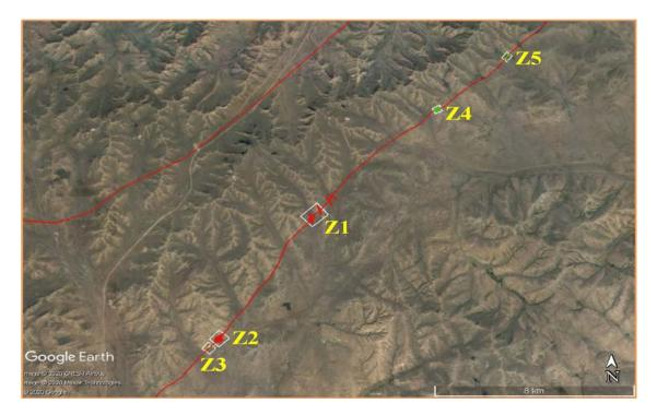
Figure 2.23 GPR survey locations map of the Avdar fault. Z1-Z2 are GPR zones surveyed in 2011. Z3 is surveyed in 2012 and Z4-Z5 are surveyed in 2016. Two red lines are Avdar fault traces.
