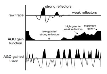
Figure 1.14 The effect of an AGC function applied to a radar trace. See (Inc., 2001; Inc, 2020).
