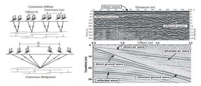
Figure 1.6 The different acquisition modes typical of ground penetrating radar, with constant offset at the top, in the CMP mode at the bottom. On the right, an example of the typical image obtained for each of the modes with the different types of arrivals indicated (Figure 1.1) after (Bano, 2000; Steelman & Endres, 2011).
