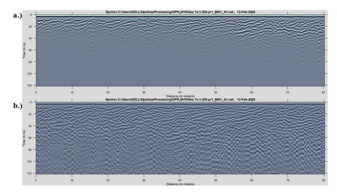
Figure 1.17 AGC processing. a) Example of GPR profile before AGC processing; b) GPR profile after AGC processing.
