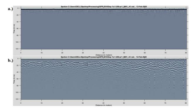
Figure 1.12 Amplification processing. a) Example of GPR profile before Amplification processing; b) GPR profile after Amplification processing.
