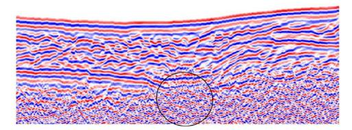
Figure 5.2 The facies used in the interpretation of the 250MHz GPR result images on the high angle normal structure zone. Clear strongly horizontal reflection layer, it is almost parallel to the surface topography. A strongly attenuated signal and don't have any reflection in the high angle vertical structure of the high angle normal structure (black circle).
