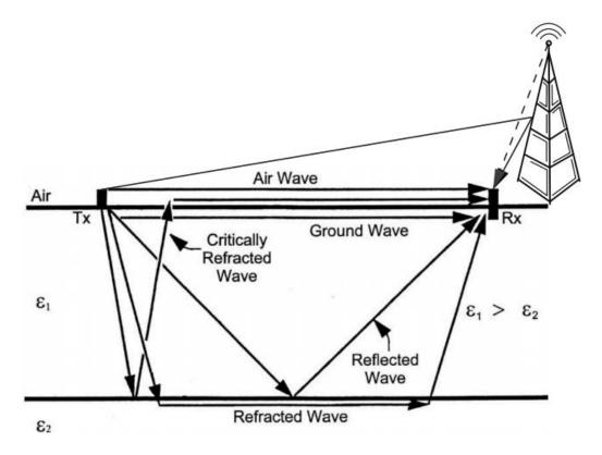
Figure 1.1 Path of propagation of electromagnetic waves in the ground in the case of a twolayer medium with contrasting dielectric permittivity ( $\varepsilon_1$  and  $\varepsilon_2$ ), after (Sperl, 1999).
