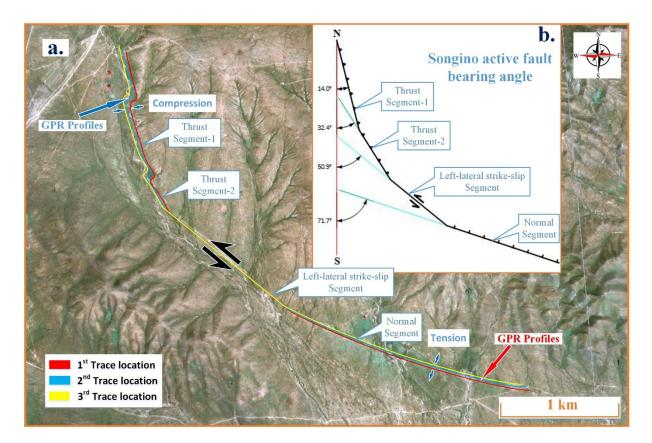
Figure 4.10 The Songino active fault modelling. a. red line indicates the  $1^{st}$  trace location of the Songino fault, Blue line represent  $2^{nd}$  trace location after  $1^{st}$  seismic event, Yellow one is  $3^{rd}$  trace location after  $2^{nd}$  seismic event. b. four different direction fault trace bearing angle and fault interpretation.
