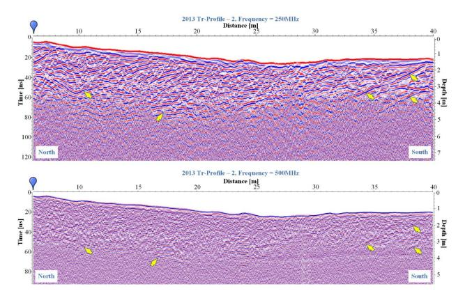
Figure 3.14 The result of GPR images of the profile P2 inside the trench (acquired the August 2013) obtained with 500MHz and 250 MHz antenna in the Songino fault study area S5 (see location in Figure 3.13). a) Result of GPR image of profile P2 obtained with 250 MHz. b) Result of GPR image of profile P2 obtained with 500 MHz antenna. The blue symbols indicate the initial position of the measurements, yellow arrows are pointing underground high reflected GPR anomalies.
