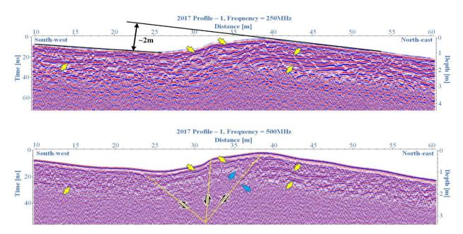
Figure 2.7 GPR result image of the Profile-1 (acquired the June 2017) interpretation of the zone 2 (back-thrust structured) of the Mogod active fault (Figure 2.6c). First figure is 250MHz antenna result image, yellow arrows show the reflections from layers. Second figure is 500 MHz antenna result image, blue arrow is same layer, orange line is strong reflected layers, black arrows indicated movement direction.
