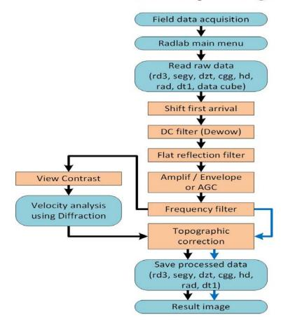
Figure 3.3 2D GPR data processing flow chart. Blue one is data input and output steps, orange one is GPR data processing steps. Black arrows following with velocity analysis, blue arrows following without velocity analysis.
