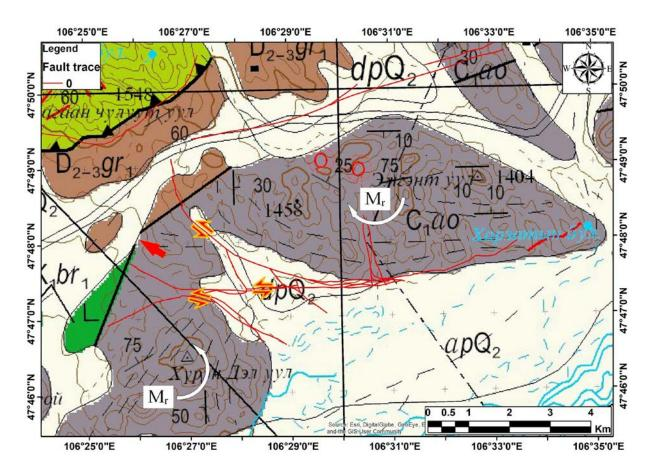
Figure 4.15 Geological background map of the Songino active fault area. Red lines indicated fault trace location of the Songino fault. Red arrow pair point to the movement directions. Mongolian Geological Map-200 project, 2005, scale 1:200 000, map number is 5732.
