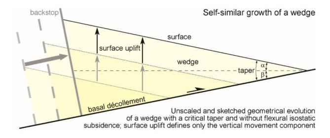
Figure 4.17 Geometry and growth of a wedge structure and bulldozer effect (Burg, 2017).
