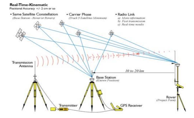
Figure 1.4 RTK and DGPS/GNSS. Source: after (Jan, 2015)
