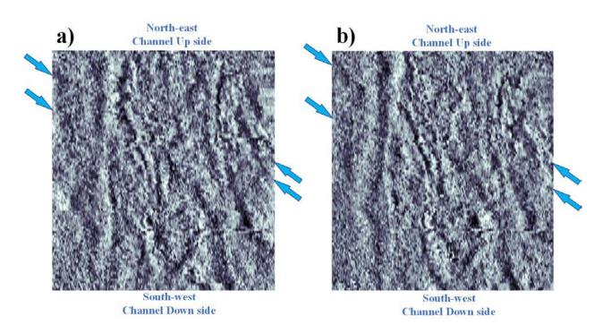
Figure 2.39 Result of depth slices images of the C1 pseudo-3D data cube (acquired the June 2010) obtained with 500 MHz shielded antenna in the paleo river channel of the Emeelt active fault. a) Depth slice 0.48 m below ground surface, b) Depth slice 0.53m below ground surface, blue arrows indicating fault traces. Channel upside is rainwater inlet side and channel downside are rainwater outlet side.
