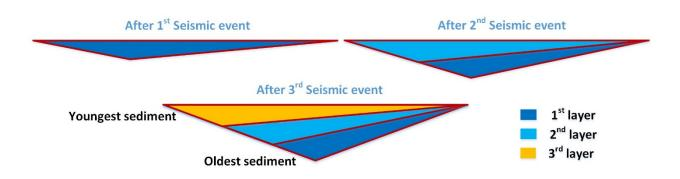
Figure 4.6 The paleo-seismological trench interpretation of sediment layered structure. The dark blue is  $1^{st}$  and oldest sediment and mud layer, the light blue is  $2^{nd}$  sediment layer and the orange one  $3^{rd}$  and youngest sediment layer. The trench photo mosaic in Figure 4.5.
