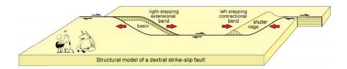
Figure 4.14 Strike slip faulting and sedimentation. This is dextral strike-slip fault example. Left side extensional zone with pull-apart oblique normal structure, Right side compressional zone with push-up oblique thrust structure (Burg, 2017).
