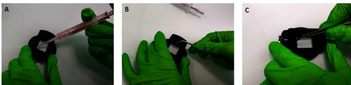
Figure 5: Sealing the DLS rotation device.
