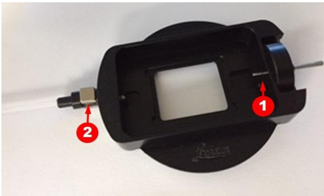
Figure 9: Placing the FEP tube in the rotation device (first step).
