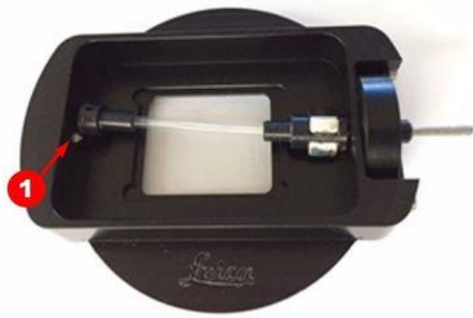
Figure 10: Placing the FEP tube in the rotation device (final step).
