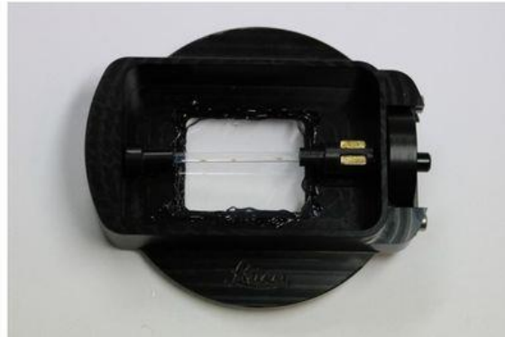
Figure 10: Placing the FEP tube in the rotation device (final step).
