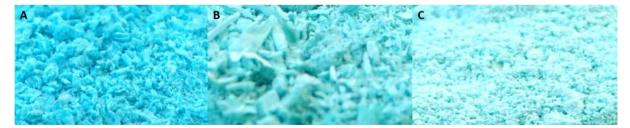
**Figure 42.** Macroscopic comparison of copper oxide precursor samples prepared at A) 130°C; B) 145°C and C) 155°C.
