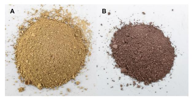
**Figure 84.** Photography of copper/titanium oxide mixture calcined at (A) 400°C and (B) 600°C.
