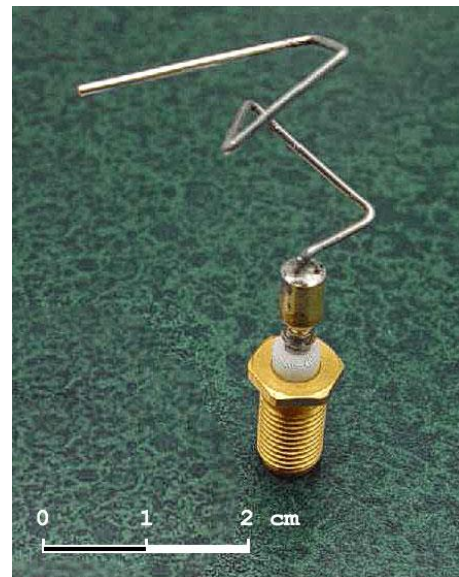
Figure 111. ST5 antenna designed using GA techniques (NASA, 2006 - public domain).
