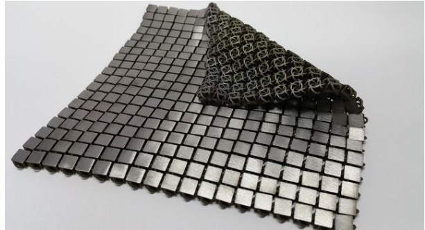
Figure 140. Multifunctional 3D printed fabric developed by the author, after JPL NASA / Caltech (2017).
