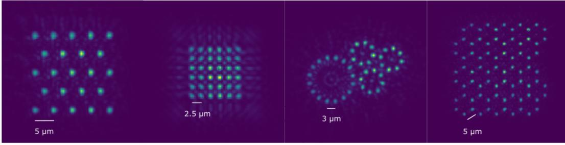
**Fig. 3.13: Intensity patterns produced by DMD.** From left to right: Triangular lattice ( $5 \times 5$ ), square lattice ( $6 \times 6$ ), the structure of light harvesting complex, Hexagonal lattice ( $6 \times 6$ ).
