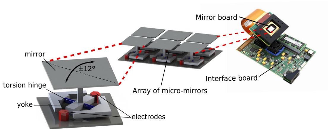
**Fig. 3.5: Schematic of DMD** Digital micromirror device where all of the  $1024 \times 768$  mirrors are situated on a rectangular mirror board of about  $1.5 \text{ cm}^2$  along with the zoomed-in part of the mirror array showing their tilt of  $\pm 12^\circ$  across the diagonal axis of the micromirror referring to the ON/OFF state of the device (Image adapted from [135, 136])
