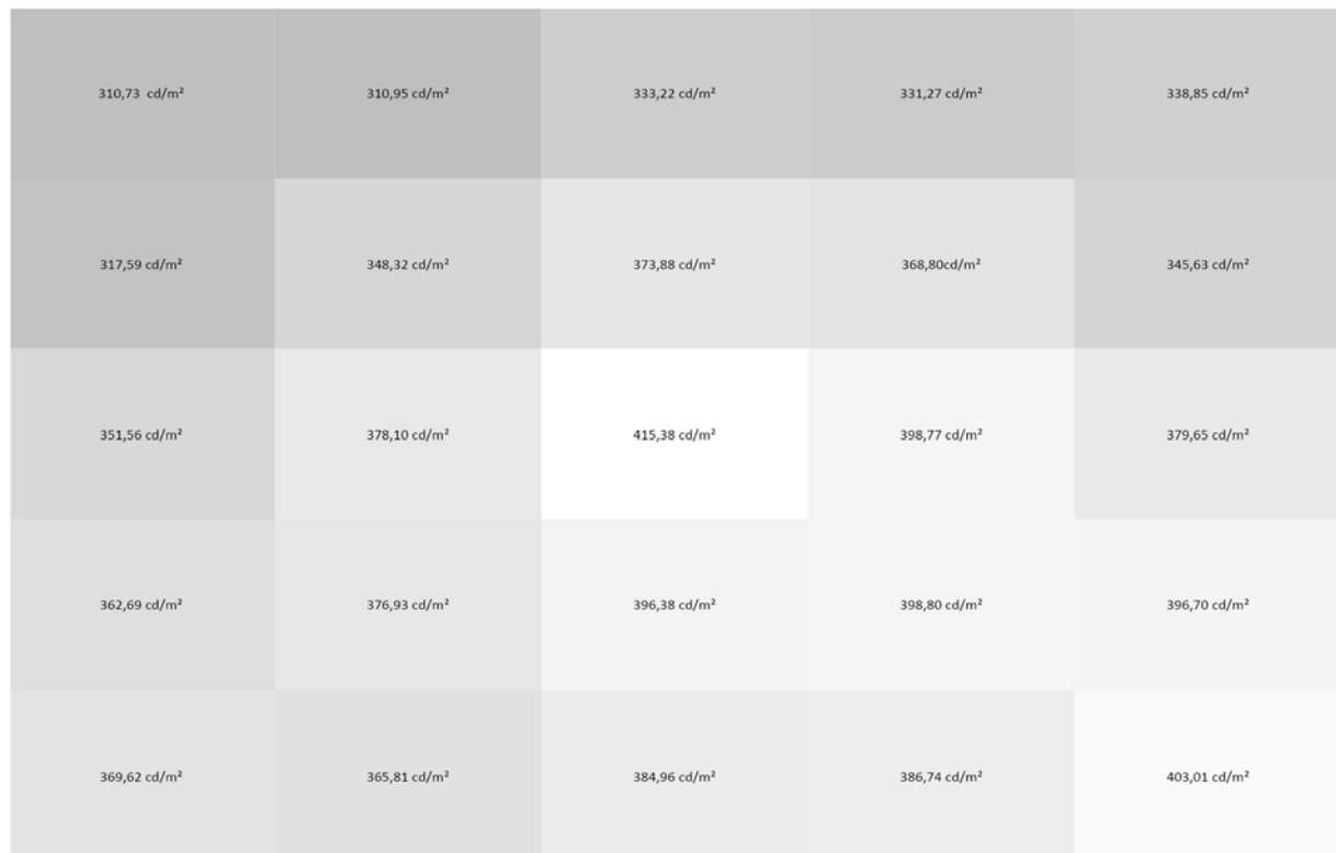
Figure 34. Visualization of the measured luminance differences at 100% for Display 1.
