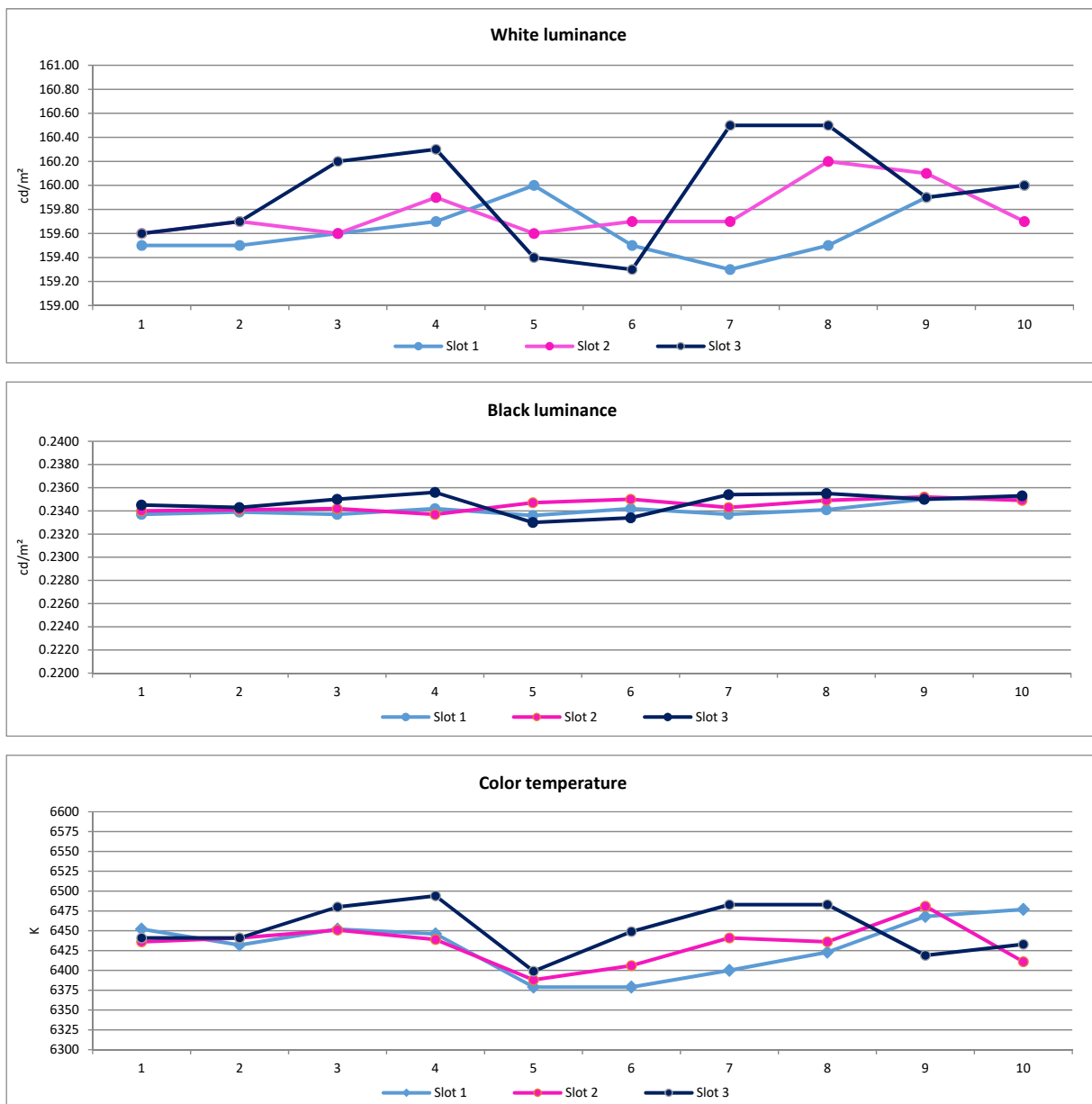
Figure 43. Measured values achieved per time slot for Display 1 (10 measurements in the test period of five days).
