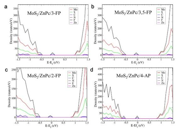
**Figure 8.10:** Density of states of  $MoS_2/ZnPc/fPys$  with (a) 3-FP, (b) 3,5-FP, (c) 2-FP, and (d) 4-AP functional groups. All  $MoS_2/ZnPc/fPy$  systems form Type II heterostructures with HOMO of the molecule (indicated at E-E<sub>f</sub> = 0 eV) forming the valence band and  $MoS_2$  surface forming the conduction band. When fPys are varied, small changes in the position of conduction band with respect to HOMO of the molecule were observed.
