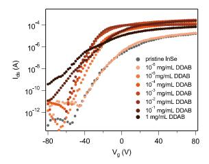
$\textbf{Figure 7.3:} \ Transfer \ (V_g\text{-}I_{ds}) \ curve \ of \ InSe \ FET \ functionalized \ with \ DDAB \ with \ different \ concentration.$
