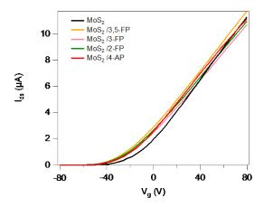
**Figure 8.8:** Control experiment of FET measurement of monolayer  $MoS_2$  only with fPys functionalization step, indicating that without MPcs serving as templating layer for the ligands, the fPys interact weakly via physisorption with  $MoS_2$ , and upon thermal annealing the pyridines desorb thereby yielding a negligible doping effect.
