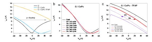
**Figure 9.8:** Control experiment of the molecular switch photoswitching on graphene FET. (a)  $I_d$ - $V_g$  curve of graphene FET before and after each step of molecular switch growth. (b)-(c) Photoswitching cycles of the molecular switch on graphene (b)before and (c) after the coordination with TFAP ligand.
