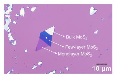
**Figure 4.4:** Optical microscope image of monolyer, few-layer and bulk MoS<sub>2</sub> on Si/SiO<sub>2</sub> (270nm) substrate.
