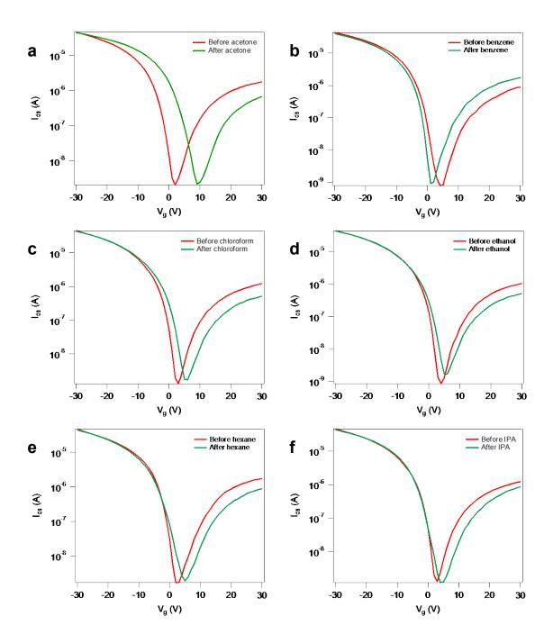
**Figure 6.4 (see also next page):** Transfer curve (logI<sub>ds</sub> vs V<sub>g</sub>) of few-layer BP before and after physisorption of (a) acetone, (b) benzene, (c) chloroform, (d) ethanol, (e) hexane, (f) IPA, (g) m-xylene, (h) p-xylene, and (h) toluene.
