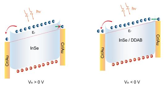
Figure 7.18: Band diagram of InSe photoFET before and after functionalization with DDAB at  $V_g=0V$ .
