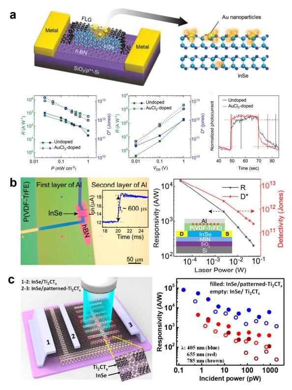
**Figure 2.15:** Photodetection enhancement of InSe. (a) AlCl<sub>3</sub> surface doped InSe photodetector. Adapted from Ref.[72] (b) Ferroelectric-gated InSe photodetector. Adapted from Ref.[73] (c) Transition metal carbide enhanced InSe photodetector. Adapted from Ref. [74]
