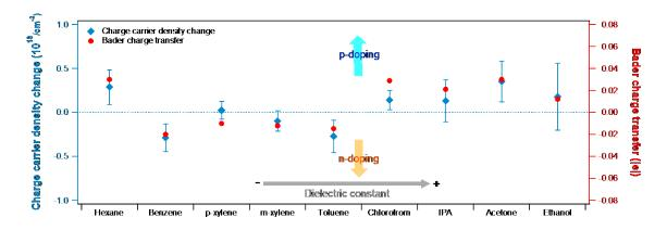
**Figure 6.7:** Charge carrier density change of BP FET after physisorption of solvent molecules and calculated Bader charge transfer in solvent-phosphorene systems.
