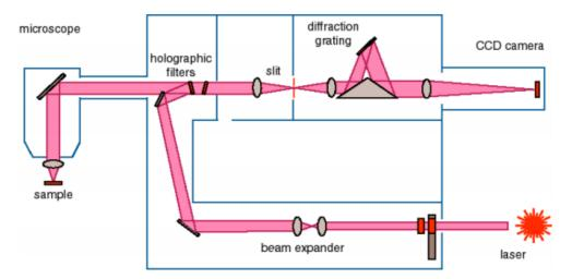
**Figure 4.21:** Schematic representation of Renishaw Raman spectrometer (Source: Renishaw Raman spectrometer Manual).
