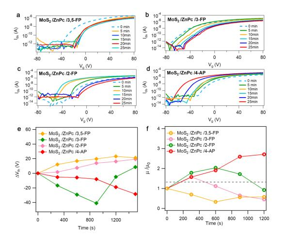
**Figure 8.7.** Kinetic analysis of MoS<sub>2</sub>/ZnPc coordinated with ligands. (a)-(d) Transfer curve of FET with different functionalization time of fPys. (e) The threshold voltage change of each functionalization time. (f) Charge carrier mobility change of MoS<sub>2</sub>/ZnPc functionalized by different fPys.
