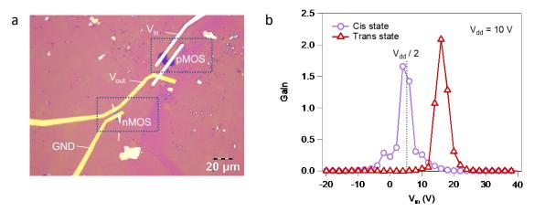
**Figure 9.13:** (a) Optical microscope image of  $MoS_2$ -WSe<sub>2</sub> inverter. (b) Voltage gain of the molecular controlled inverter at unfolded state and folded state of the molecular switch. The overall gain is smaller than in previously reported work because of the use of relatively low-k dielectric material (SiO<sub>2</sub>).
