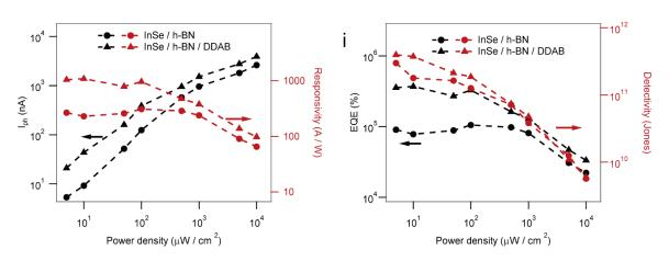
**Figure 7.34:** Power dependence of (a) photocurrent and responsivity and (b) EQE and  $D^*$  of InSe/h-BN InSe/h-BN/DDAB on BCB at  $V_g$ =0V and  $V_d$ =1V illuminated with 365 nm light.
