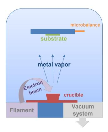
**Figure 4.12:** Illustration of the Ebeam evaporation mechanisms.
