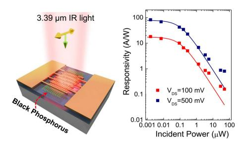
**Figure 2.10:** Black phosphorus mid-infrared (MIR) photodetector. Left: Demonstration of device structure. Right: Photoresponsivity of BP photodetector under different light power. Adapted from Ref.[48]
