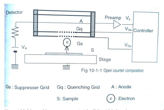
**Figure 4.25:** Scheme of the measurement principle of Riken AC-2 photoelectron spectrometer. (Source: RIKEN KEIKI CO.,LTD)
