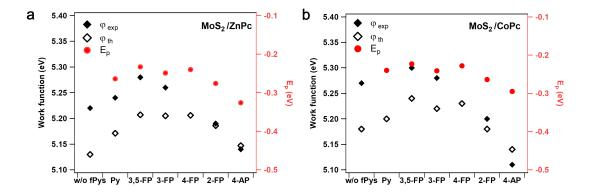
**Figure 8.12:** Calculated work function of MoS<sub>2</sub>/MPc/fPys for (a) M=Zn, and (b) M=Co. The  $\phi_{exp}$  stands for experimental work function values measured by PhotoElectron Yield counter operating in Ambient conditions (PEYA) which are presented in **Figure S8**. The work function trends follow the computed dipole induced electrostatic potential (E<sub>p</sub>) of the isolated molecules at vacuum level.
