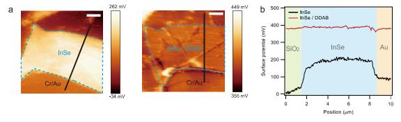
**Figure 7.5:** (a) Surface potential measured by Kelvin probe force microscopy (KPFM) of few-layer InSe of before and after functionalization with DDAB (scale bar: 3 @m) and (b) the corresponding line potential profile of marked in black line in (a).
