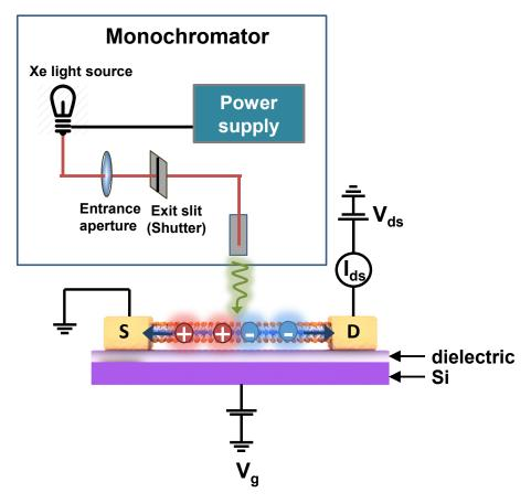
Figure 4.19: Schematic representation of the photodetector measurement.
