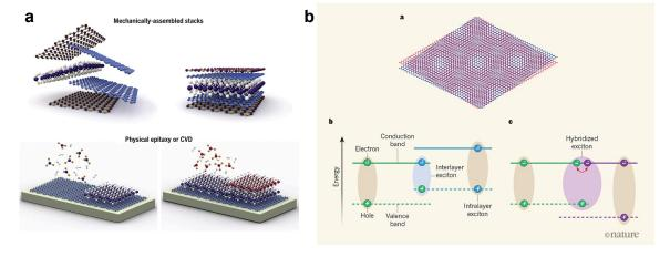
**Figure 2.16:** Stacking of van der Waals (vdW) heterostructures. (a) Mechanical assembling of 2D heterostructures and direct epitaxy and CVD growth of heterostructures. Adapted from Ref.[79] (b) Moiré heterostructures and its optical properties. Adapted from Ref.[78]
