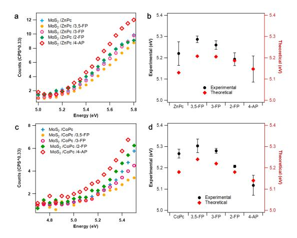
**Figure 8.14:** Work function plots of (a)  $MoS_2/ZnPc/fPys$  and (c)  $MoS_2/MPc/fPys$  measured by PhotoElectron Yield counter operating in Ambient conditions (PEYA). For the sake of comparison, work function values of (b)  $MoS_2/ZnPc/fPys$ , and (d)  $MoS_2/MPc/fPys$  computed by DFT calculations are also depicted.
