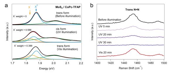
**Figure 9.11:** Optical properties of MoS<sub>2</sub> controlled by molecular switch. (a) Photoluminescence (PL) spectra of molecular switch on monolayer MoS<sub>2</sub> modulated by light illumination. (b) High wavenumber range of Raman spectra of molecular machine on monolayer MoS<sub>2</sub> modulated by light illumination. The trans-azo feature is present at 1450 cm<sup>-1</sup>, the peak disappeared progressively by UV illumination and recovers by the Vis illumination.
