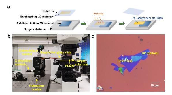
**Figure 4.5:** Dry transfer of 2D heterostructures. (a) Schematic demonstration of PDMS-assisted dry transfer. (b) Photo of the experimental setup for dry transfer which contains an optical microscope and a home-made transfer setup. (c) Optical microscope image of transferred heterostructures in which BP was firstly exfoliated onto the  $Si/SiO_2$  substrate and InSe was transferred onto the substrate to partially cover the BP flake by PDMS.
