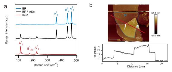
Figure 7.39: (a) Raman spectra and (b) AFM height image of as fabricated heterostructure.
