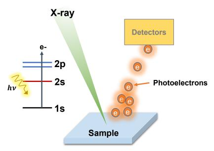
**Figure 4.23:** Mechanism of photoelectron generation and the schematic representation of XPS instrument.
