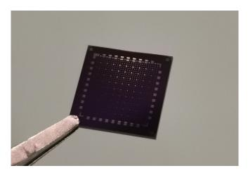
**Figure 4.1:** Photo of pre-patterned Si/SiO<sub>2</sub> (270 nm) substrate for fabricating optoelectronic devices based on 2D materials.
