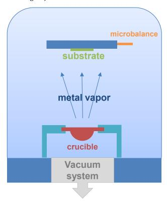
**Figure 4.11:** Illustration of the thermal evaporation mechanisms.
