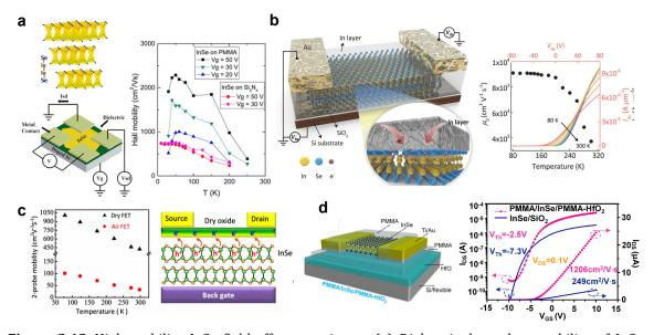
**Figure 2.13:** High mobility InSe field-effect transistors. (a) Dielectric-dependent mobility of InSe. Adapted from Ref.[64] (b) High electron mobility by indium encapsulation. Adapted from Ref.[65] (c) Surface oxide mediated high mobility of InSe. Adapted from Ref.[62] (d) Polymer-encapsulated high-mobility InSe FET. Adapted from Ref.[66]
