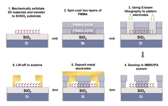
Figure 4.9: Process flow of E-beam lithography.
