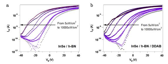
**Figure 7.35:** Gate dependent photoresponse illuminated by 365 nm light of InSe Schottky junction. Transfer curve (a) before, and (b) after doping with DDAB. with light power ranging from 5  $\mu$ W/cm<sup>2</sup> to 10000  $\mu$ W/cm<sup>2</sup>.
