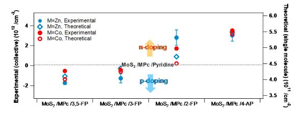
**Figure 8.6:** Charge carrier density shift in monolayer MoS<sub>2</sub> after ligand functionalization of fPys on MPc obtained from FET measurements with comparison to the theoretical results calculated from work function analysis.
