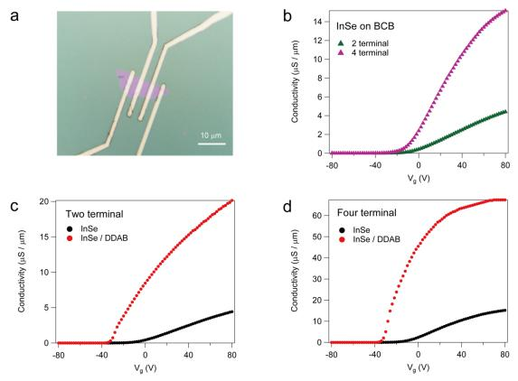
**Figure 7.15.** Four-terminal measurement of InSe with Cr/ Au contact. (a) Optical image of few-layer InSe device with four terminals. The gap between two adjacent terminals amount to 3.5  $\square$ m. (b) Typical comparison of gate-dependent conductance of two-terminal and four-terminal measurements at V<sub>ds</sub>=1V. (c)-(d) Comparison of gate-dependent conductance of InSe and InSe/DDAB obtained from (c) two-terminal and (d) four terminal measurements.
