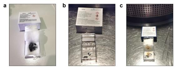
**Figure 4.2:** Bulk crystals of (a) MoS<sub>2</sub>, (b) InSe and (c) black phosphorus (BP). Due to the chemical instability of InSe and BP in air, the bulk crystals are stored in a nitrogen-filled glovebox with oxygen and water level below 1 ppm.
