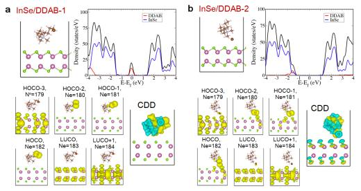
**Figure 7.9:** Atomic positions and electronic structure of InSe/DDAB heterostructures for DDAB adsorbed on pristine InSe surface. Atomic positions (optimized geometry) and electronic structure of InSe/DDAB heterostructures for DDAB adsorbed on pristine InSe surface when (a) Br atom is farther away from the basal plane of InSe: Conformation-1 and (b) Br atom is closer to the basal plane of InSe:
