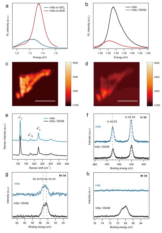
**Figure 7.16:** Spectroscopic characterization of functionalized InSe. (a) Photoluminescence spectra of InSe on  $SiO_2$  and BCB substrate. (b) Photoluminescence spectra of InSe without and with DDAB functionalization. PL mapping of InSe (c) before and (d) after functionalization with DDAB. The scale bar is 10  $\mathbb{Z}$ m. e, Raman spectra of InSe and InSe/DDAB. High resolution XPS spectra of (f) In 3d, (g) Se 3d, and (h) Br 3d of InSe and InSe/DDAB.
