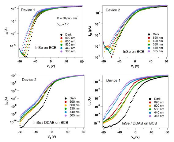
**Figure 7.20:** Photoresponse of two others representative InSe photoFETs before and after doping with DDAB. All devices yield statistically similar behavior upon molecular doping and photoresponse, including the devices shown in **Figure 7.17**.
