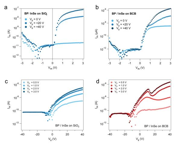
**Figure 7.41:** Detailed electrical performances of BP-InSe heterostructure on different substrates. Gate-dependent output characteristics (a) SiO<sub>2</sub> and (b) BCB. Drain-bias-dependent transfer curves of BP-InSe heterostructure on (c) SiO<sub>2</sub> and (d) BCB.
