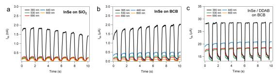
**Figure 7.19:** Time-resolved photoresponse cycles. Photoresponse curves of different wavelength of (a) InSe on SiO<sub>2</sub>, (b) InSe on BCB, (c) InSe/DDAB on BCB. The incident light power is adjusted to 34.3 mW/cm<sup>2</sup> for each wavelength.
