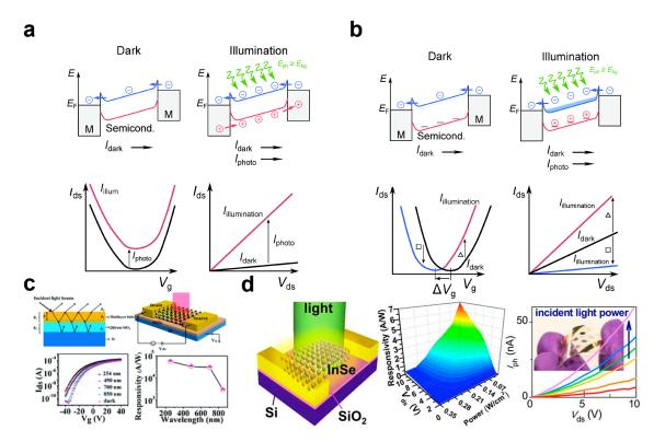
**Figure 2.14:** Indium selenide photodetectors. (a) Illustration of mechanism of photoconductive effect. Adapted from Ref. [67] (b) Illustration of mechanism of photogating effect. Adapted from Ref. [67] (c) InSe photodetectors on  $Si/SiO_2$  substrate. Adapted from [68] (d) InSe photodetectors on  $Si/SiO_2$  substrate and on flexible substrate. Adapted from Ref. [69].
