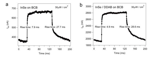
**Figure 7.25:** Time response of low-power light illumination. Photoresponse at 365 nm of (a) InSe on BCB, and (b) InSe/DDAB on BCB.
