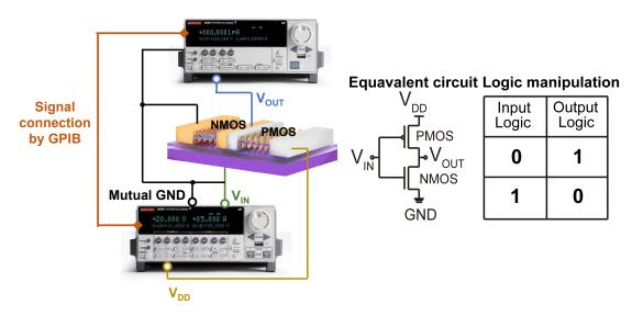
**Figure 4.20:** Schematic illustration of logic inverter measurement setup, the equivalent circuit and logic manipulation.
