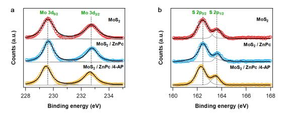
**Figure 8.2:** XPS (a) Mo 3d and (b) S 2p spectra of MoS<sub>2</sub>/ ZnPc hybrid functionalized with 4-AP.
