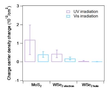
**Figure 9.7:** Statistical analysis of charge carrier density modulation of MX<sub>2</sub>/CoPc-TFAP by UV and Vis irradiation.
