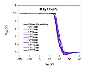
**Figure 9.14:** Vout-Vin of the inverter ( $MX_2$ / CoPc) without the TFAP ligand. The inverter did not show distinct transition point shift with light illumination, indicating that the dynamic modulation is merely caused by the motion of TFAP ligand.
