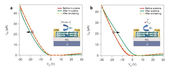
**Figure 6.1:** Typical transfer curve of few-layer black phosphorus field-effect transistor before and after physisorption of (a) m-xylene, and (b) acetone.
