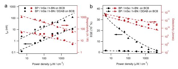
**Figure 7.52:** Power dependence of (a) photocurrent and responsivity and (b) EQE and  $D^*$  of BP/InSe/h-BN and InSe/h-BN/DDAB at  $V_g$ =V and  $V_d$ =1V illuminated with 365 nm light.
