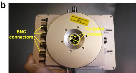
**Figure 4.22:** Low-temperature Photoluminescence and Raman measurement. (a) Photo of Linkam temperature controlling TMHS600 stage equipped onto Renishaw Raman spectrometer. (b) Photo of Linkam HFS600E-PB4 with probes and BNC connectors.
