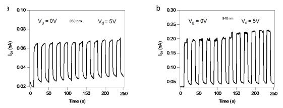
**Figure 7.32.** Photoresponse of lateral InSe Schottky junction illuminated at near-infrared (NIR) region. Time dependent photoresponse at  $V_d$ =5V and  $V_g$ =0V for illumination at (a) 850 nm and (b) 940 nm.
