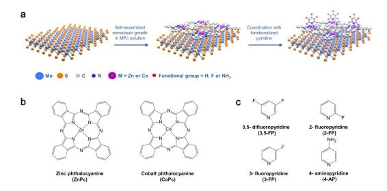
**Scheme 8.1.** (a) Illustration of two-step functionalization of ligand-coordinated MoS<sub>2</sub>/MPc heterojunction. Chemical structure of (b) MPcs and (c) fPys used in this work.
