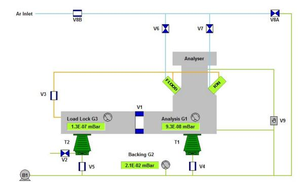
Figure 4.24: Scheme of the Thermo Fischer XPS instrument used in this thesis.
