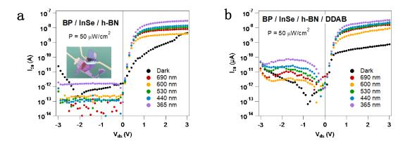
**Figure 7.49:** Light responsive output curves of another representative BP/InSe vdW P-N heterostructure. (a) Output curve before DDAB functionalization. (b) output curve after DDAB functionalization.
