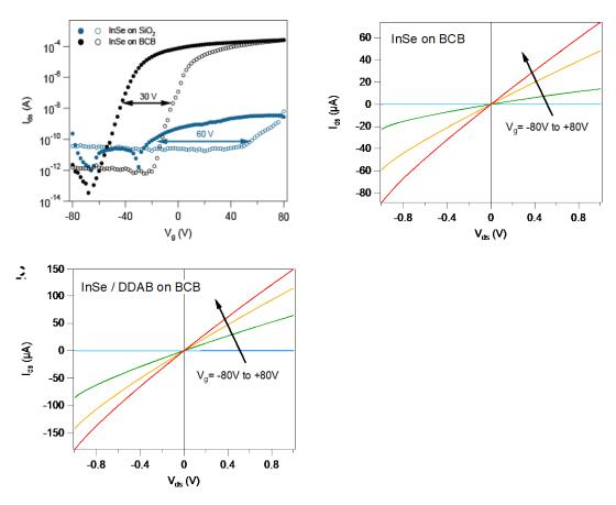
**Figure 7.2:** Current-voltage characteristics of InSe FETs. (a) Comparison of the hysteresis of InSe FET on  $SiO_2$  and BCB. A decrease of 30V is observed after the dielectric engineering. The presence of 30V of hysteresis is attributed to the surface oxide of InSe in the chemical form of  $InO_x$  unintentionally introduced during the nanofabrication which acts as charge traps.[62,63,189,190] Gate –dependent output curves of InSe (b) before and (c) after doping with DDAB.
