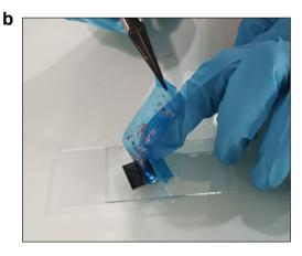
**Figure 4.3:** Mechanical exfoliation of 2D materials. (a) Examples of exfoliated materials (MoS<sub>2</sub>) on different materials. (b) Transfer of exfoliated flakes onto Si/SiO<sub>2</sub> substrate.
