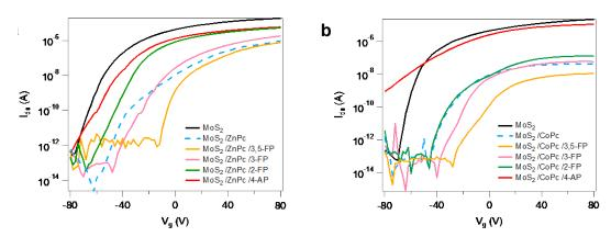
**Figure 8.4:** (a) Comparison of transfer curves of MoS<sub>2</sub>/ZnPc heterojuction coordinated with ligands. (b) Comparison of transfer curves of MoS<sub>2</sub>/CoPc heterojuction coordinated with ligands.
