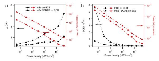
**Figure 7.23:** Power dependence of (a) photocurrent and responsivity and (b) EQE and detectivity of InSe on SiO<sub>2</sub>, InSe on BCB and InSe/DDAB on BCB at  $V_g$ =0V and  $V_{ds}$ =1V illuminated with 365 nm light.
