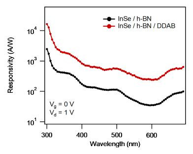
**Figure 7.31:** Calculated responsivity with of lateral InSe Schottky junction. Responsivity with wavelength scan from 300 nm to 690 nm. The interval of wavelength is 5 nm.
