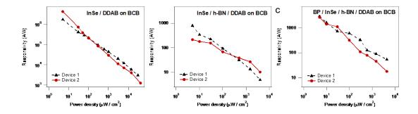
**Figure 7.53:** Statistical analysis of the photoresponsivity of additional devices. Plots of responsivity versus power density of DDAB functionalized devices of (a) InSe phototransistor, (b) InSe lateral Schottky diode, (c) BP/InSe vertical vdW PN heterojunction.
