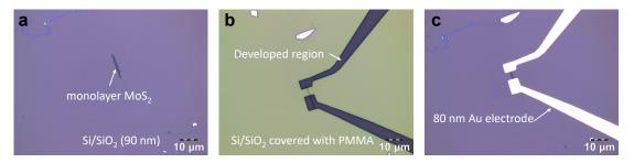
**Figure 4.13:** Optical microscope image of each step of the monolayer MoS<sub>2</sub> field-effect transistor: (a) Before lithography; (b) After development; (c) After lift-off.
