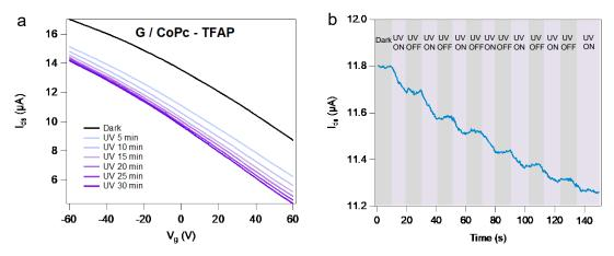
**Figure 9.9:** Time-dependent doping of graphene by molecular switch. (a) Transfer curve of G/CoPc-TFAP FET of different UV illumination time. (b) Time-dependence Ids at  $V_g=0$  V with 10s UV pulse cycles of G/CoPc-TFAP FET.
