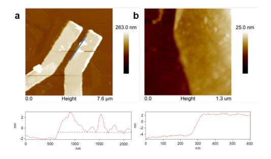
**Figure 6.2:** Topographical AFM image of a BP FET device with flake thickness of (a)  $\sim$ 2.5 nm, and (b)  $\sim$ 6.5 nm. The hills in the height profile are caused by rapid degradation occurred when measuring in air.
