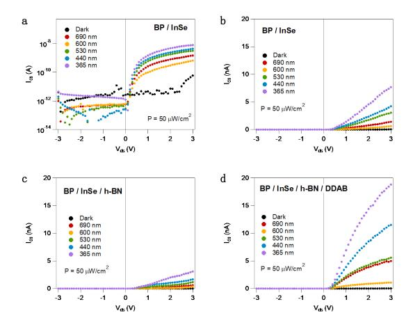
**Figure 7.47:** Other photoresponse characteristics of BP-InSe heterostructure. (a) Output curve of BP/InSe on BCB before encapsulation with h-BN of the specific device shown in Figure 7.4. Output curves of (b) BP/InSe (c) BP/InSe/h-BN (d) BP/InSe/h-BN/DDAB plotted in linear scale.
