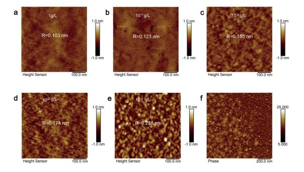
**Figure 7.14:** AFM images of DDAB on InSe. High resolution AFM height image of InSe functionalized by spin-coating a solution of DDAB molecule in tetrachloroethane (TCE) of the following concentrations (a) 1 g/L; (b)  $10^{-1}$  g/L; (c)  $10^{-2}$  g/L; (d)  $10^{-4}$  g/L; (e)  $10^{-5}$  g/L. (f) AFM phase image of InSe functionalized via spin-coating a  $10^{-5}$  g/L solution of DDAB.
