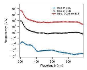
**Figure 7.21:** Calculated responsivity with of wavelength scan from 300 nm to 690 nm at high incident light power (34.3 mW/cm<sup>2</sup> for 365 nm light). The interval of wavelength is 5 nm.
