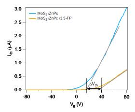
**Figure 8.5:** Typical transfer curve of MoS<sub>2</sub>/ZnPc and MoS<sub>2</sub>/ZnPc/3,5-FP showing the calculation of  $\Delta V_{th}$  before and after ligand functionalization.
