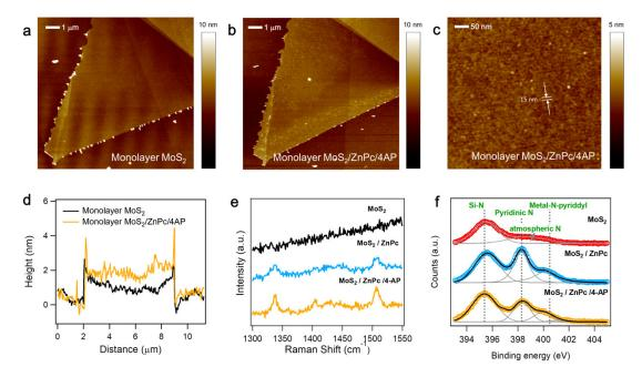
**Figure 8.1:** Surface characterizations of  $MoS_2/ZnPc/4$ -AP. Topographic AFM image of (a) pristine monolayer  $MoS_2$  and (b) monolayer  $MoS_2/ZnPc/4$ -AP, (c) the latter also on the sub- $\mu$ m scale. (d) Height profile of monolayer  $MoS_2$  and monolayer  $MoS_2/ZnPc/4$ -AP. (e) Raman spectra of monolayer  $MoS_2$ , monolayer  $MoS_2/ZnPc/4$ -AP in high wavenumber range. (f) XPS spectra of N 1s of monolayer  $MoS_2$ , monolayer  $MoS_2/ZnPc/4$ -AP.
