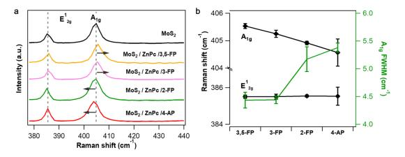
**Figure 8.18:** (a) Raman spectra of pristine  $MoS_2$  and functionalized with ZnPc/fPys. (b) Plot of the shift in  $E^1_{2g}$  mode and  $A_{1g}$  mode, and the variation of full width of half maximum (FWHM) of  $A_{1g}$  peak upon the functionalization by different fPy ligands.
