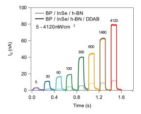
**Figure 7.51:** Photoresponse of power density ranging from  $5\mu W/cm^2$  to  $4120\mu W/cm^2$  of BP/ InSe/h-BN and BP/ InSe/h-BN/DDAB.
