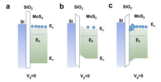
**Figure 4.16:** Band diagram of the  $MoS_2$  FET with the control of (a) zero, (b) negative and (c) positive gate voltages. Here the gate electrode is Si and the oxide is  $SiO_2$  (dielectric constant- 3.9).
