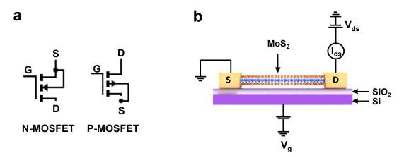
**Figure 4.15:** Electronic configuration of 2D field effect transistors. (a) Electronic symbol of N-MOSFET and P-MOSFET. (b) Device architecture of a monolayer MoS<sub>2</sub> FET.
