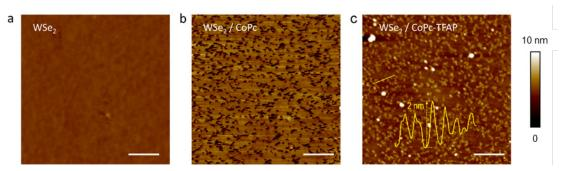
**Figure 9.4:** Surface morphology of molecular switch on the surface of WSe<sub>2</sub>. High resolution AFM image of (a) pristine WSe<sub>2</sub>, (b) WSe<sub>2</sub>/CoPc and (c) WSe<sub>2</sub>/CoPc-TFAP. The lateral scale bar is 200 nm.
