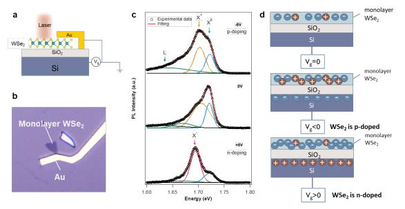
**Figure 5.16**: Gate-induced photoluminescence of monolayer WSe<sub>2</sub>. (a) Schematic representation of the device for gate-induced photoluminescence in monolayer WSe<sub>2</sub>, and (b) its corresponding optical image. (c) PL spectra of monolayer WSe<sub>2</sub> at 78 K under -5, 0, +5V, demonstrating the recombination of
