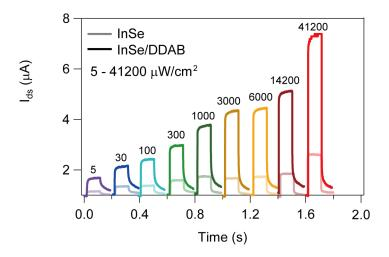
**Figure 7.24:** Time-dependent photoresponse of power density ranging from  $5 \,\mu\text{W/cm}^2$  to  $41.2 \,\text{mW/cm}^2$  of InSe and InSe/DDAB on BCB.
