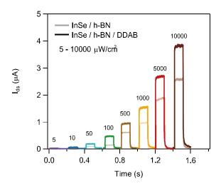
**Figure 7.33:** Time-dependent photoresponse of power density ranging from  $5\mu W/cm^2$  to  $5000\mu W/cm^2$  of InSe/h-BN and InSe/h-BN/DDAB.
