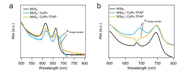
**Figure 9.6:** UV-Vis spectra of molecular switch on  $MX_2$  on sapphire. (a) UV-Vis absorption of CoPc and CoPc-TFAP on CVD monolayer  $MoS_2$ . (b) UV-Vis absorption of CoPc and CoPc-TFAP on CVD monolayer  $WSe_2$ . Additional charge transfer peak appears at 680 nm and 700 nm between CoPc complex and  $MoS_2$ , and  $WSe_2$ , respectively.
