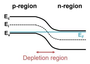
Figure 4.18: Band diagram of PN junction.
