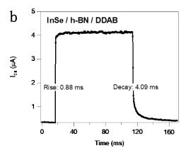
**Figure 7.36:** Time-resolved photoresponse of InSe Shottky junction. Time-resolved photoresponse of InSe Shottky junction (a) InSe/ h-BN, and (b) InSe/ h-BN/ DDAB at  $V_g$ =0V and  $V_{ds}$ =1V under the illumination of 365 nm. Light power is adjusted at 10  $\mu$ W/cm<sup>2</sup>.
