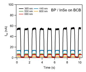
**Figure 7.44:** Time-resolved photoresponse cycles of BP/ InSe on BCB at  $V_g$ =0V and  $V_{ds}$ =1V under the illumination of 365 to 694 nm range (light power = 34.3 mW/cm<sup>2</sup>).
