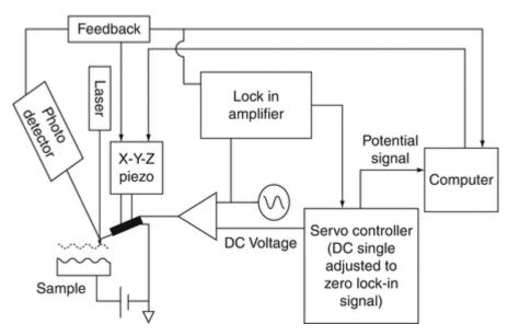
**Figure 4.26:** Schematic representation of the KPFM scan.
