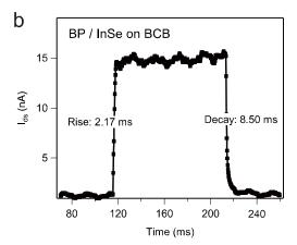
**Figure 7.43:** Time-resolved photoresponse of BP/ InSe on (a)  $SiO_2$  and (b) BP/ InSe on BCB at  $V_g$ =0V and  $V_{ds}$ =1V under the illumination of 365 nm. Light power is adjusted at 8.32 mW/cm<sup>2</sup>.
