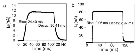
**Figure 7.48:** Time-resolved photoresponse of (a) BP/ InSe/ h-BN and (b) BP/ InSe/ h-BN/ DDAB at  $V_g$ =0V and  $V_d$ =1V under the illumination of 365 nm. Light power is adjusted at 4.12 mW/cm<sup>2</sup>.
