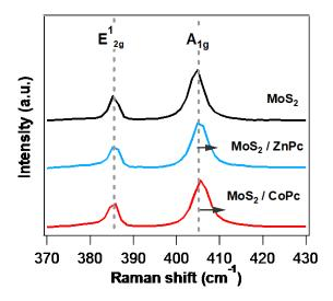
**Figure 8.17:** Raman spectra of  $MoS_2/ZnPc$  and  $MoS_2/CoPc$  compared with bare  $MoS_2$  showing a slight blueshift in  $A_{1g}$  peak and no shift in  $E^{1}_{2g}$  peak.
