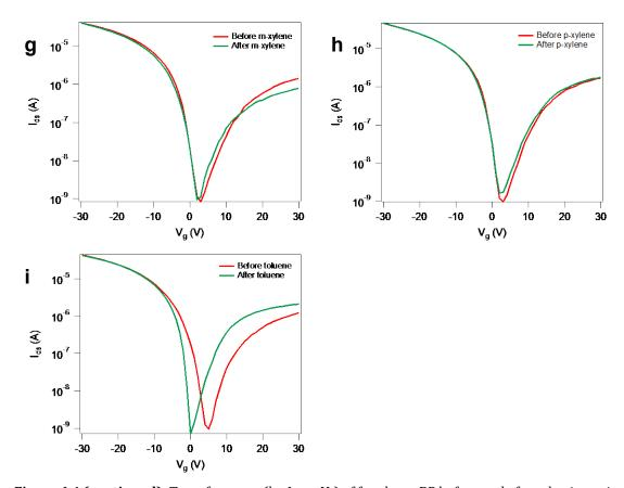
**Figure 6.4 (continued):** Transfer curve ( $logI_{ds}$  vs  $V_g$ ) of few-layer BP before and after physisorption of (a) acetone, (b) benzene, (c) chloroform, (d) ethanol, (e) hexane, (f) IPA, (g) m-xylene, (h) p-xylene, and (h) toluene.
