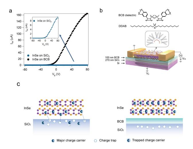
**Figure 7.1:** Dielectric engineering of few-layer InSe. (a) Comparison of transfer ( $V_g$ - $I_{ds}$ ) curve of InSe FET onto SiO<sub>2</sub> and BCB. The inset shows the zoom of transfer curve on SiO<sub>2</sub>. (b) Illustration of device structure and the chemical structure of BCB polymer and DDAB molecule used in this work. (c) Scheme of the mechanism of charge transport enhancement of InSe on SiO<sub>2</sub> and BCB.
