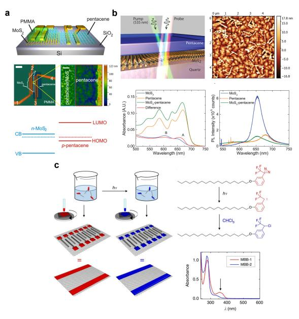
**Figure 2.17:** 2D-organic van der Waals (vdW) heterostructures. (a) P-N heterostructures formed by MoS<sub>2</sub> and pentacene. Adapted from Ref.[83] (b) Charge transfer excitons in MoS<sub>2</sub>-pentacene heterostructure. Adapted from Ref.[84](c) Periodic potential in heterostructure of graphene and self-assembled molecular layer. Adapted from Ref.[80]
