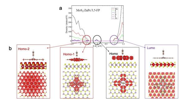
Figure 8.11: (a) Density of states, and (b) electron wavefunction plots of  $MoS_2/ZnPc/3,5$ -FP at  $\Gamma$ -point. While  $MoS_2$  surface contributes to the conduction band (indicated by wavefunction plot at LUMO), the localization of wave function on the ZnPc/3,5-FP molecules close to the Fermi energy (indicated at E-  $E_f = 0$  eV) could be observed.
