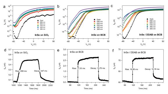
**Figure 7.17:**  $I_{ds}$ - $V_g$  curve of (a) InSe on  $SiO_2$ , (b) InSe on BCB and (c) InSe/DDAB on BCB at  $V_g$ =0V and  $V_{ds}$ =1V. Time-resolved photoresponse of (d) InSe on  $SiO_2$ , (e) InSe on BCB and (f) InSe/DDAB on BCB under the illumination of 365 nm at 34.3 mW/cm<sup>2</sup>.
