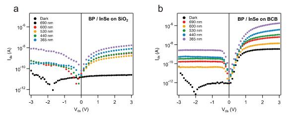
**Figure 7.40:** Output characteristic of BP-InSe heterostructure at  $V_g$ = 0V on dielectric material (a) SiO<sub>2</sub> and (b) BCB/SiO<sub>2</sub>.
