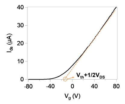
**Figure 4.17:** Representative transfer curve of monolayer  $MoS_2$  showing the extrapolation of  $V_{th}$  through the linear region.
