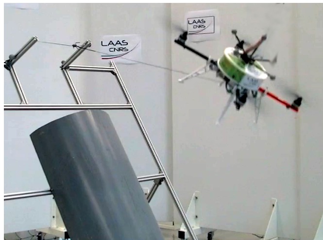
Figure 1.8 – Tethered UAV (Tognon & Franchi, 2017).
