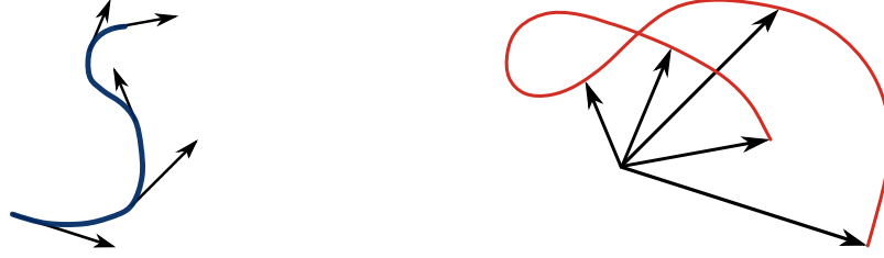
(a) A planar curve (blue) and its tangent vectors. (b) The hodograph (red) of the curve.
