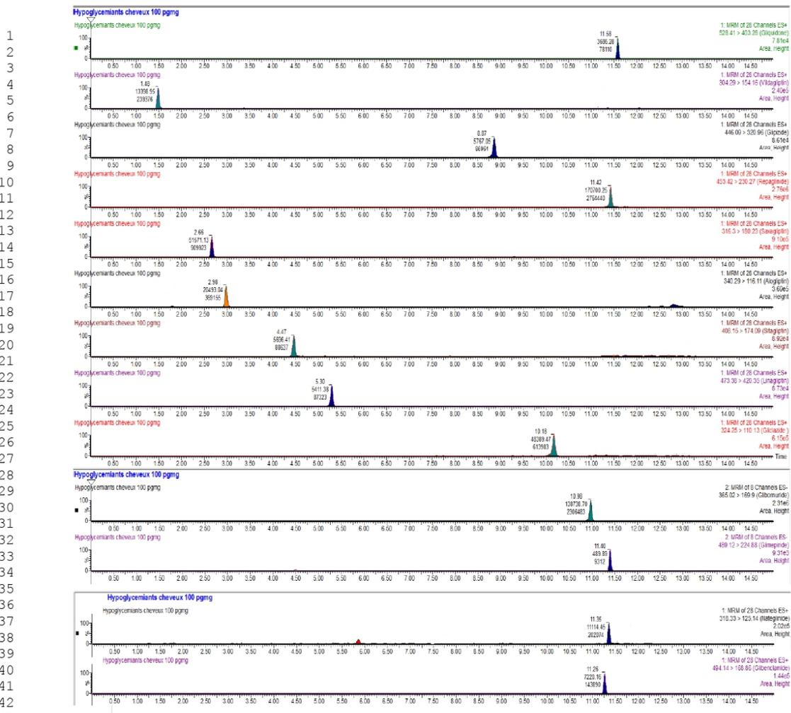
**Figure 2. Chromatograms of the ion transitions of real hair samples containing a) 2 transitions of gliclazide and 1 transition of the IS (hydroxy tolbutamide-d9), the concentration was 132 pg/mg; b) 2 transitions of sitagliptin and 1 transition of the IS (vildagliptin-d3), the concentration was 2 pg/mg; c) 2 transitions of vildagliptin and 1 transition of the IS (vidagliptin-d3), the concentration was 3 pg/mg; d) 2 transition of**
