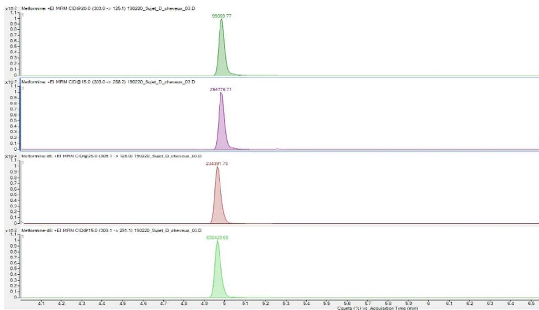
**FIGURE 1** Chromatogram of subject's hair on daily treatment, 0–2 cm (from top to the bottom: 2 transitions of metformin and 2 transitions for IS metformin-d6). Concentration was 0.3 ng/mg [Colour figure can be viewed at [wileyonlinelibrary.com](http://wileyonlinelibrary.com)]
