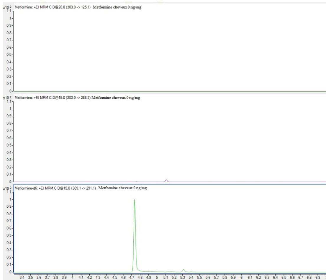
**FIGURE 2** Chromatogram of blank hair sample (from top to the bottom: 2 transitions of metformin and 1 transitions for IS metformin-d6) [Colour figure can be viewed at [wileyonlinelibrary.com](http://wileyonlinelibrary.com)]
