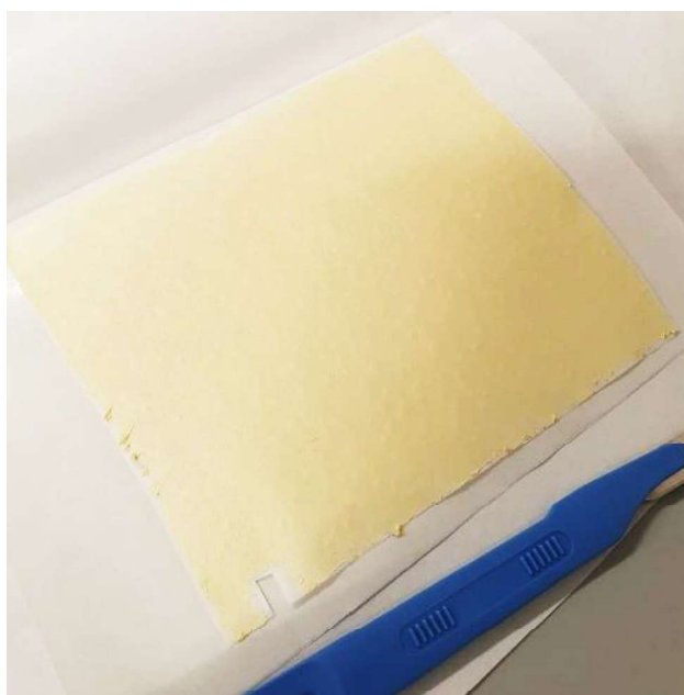
Figure 4.24. Typical appearance of nanofibrous mats containing pure [c2]daisy chain rotaxane polyurea 85a .
