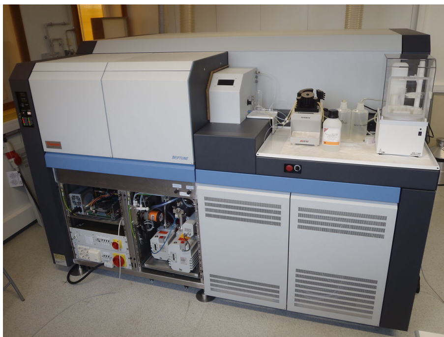
FIGURE 2.4 – Photography of the (MC-ICP-MS) Neptune Thermo Scientific instrument (photography from ITES website).
