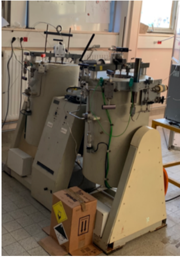
FIGURE 1.17 – Photography of the large volume autoclave, personal photography.
