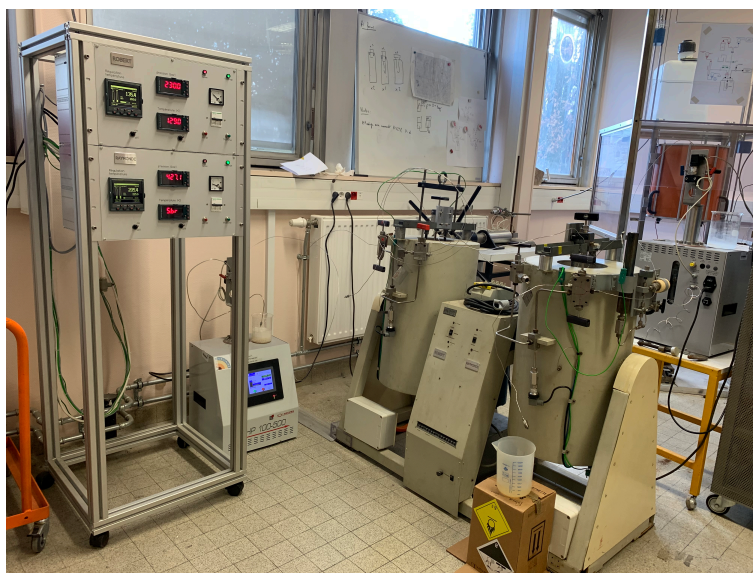
FIGURE 2.10 – Photography of the experimental setup used in this thesis. In this picture is represented the temperature and pressure command (in the left) and the two autoclaves used (i.e., Robert and Raymonde) are in the center (personal photography).
