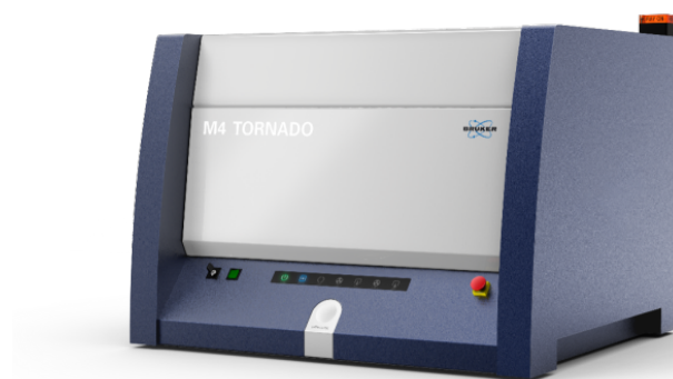
FIGURE 2.3 – Photography of the M4 tornado used for \mu XRF measurements (photography from ICube website).
