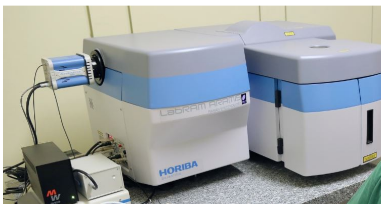
FIGURE 2.2 – Photography of the HORIBA LabRAM ARAMIS spectrometer used for the Raman analyses (photography from ICube website).
