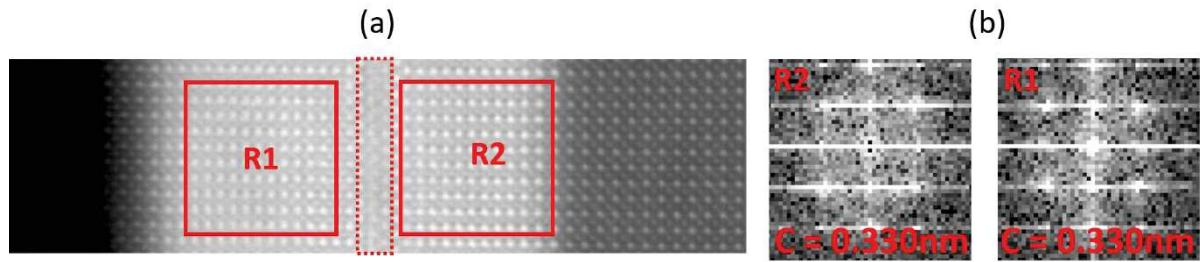
Figure IV-18 (a) STEM image of a 10 nm thick NSNO 2 (0) uncapped thin film (b) FFT of the 2 regions indicated by red boxes in (a) exhibiting c-axis parameter of 0.330 nm for both regions.
