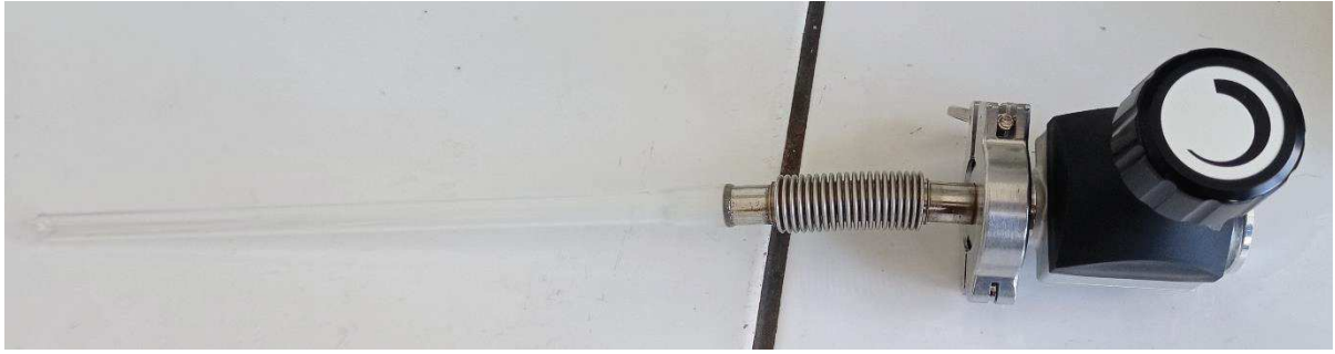
Figure III-2 Homemade system to perform the topotactic reduction of the thin films with \text{CaH}_2 powder in a static vacuum
