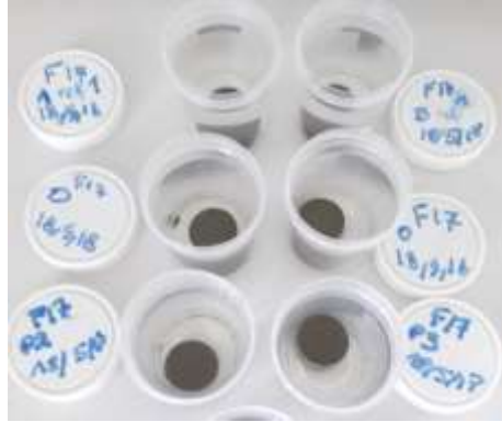
Figure 48 Cement paste sample in the acetone
