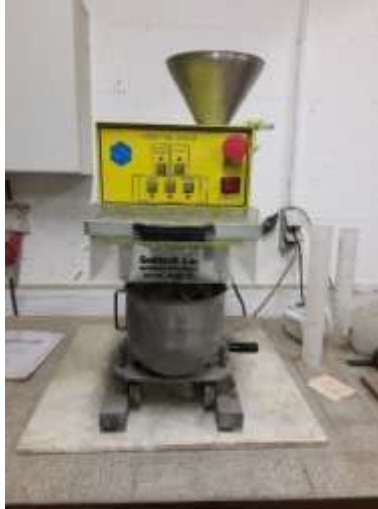
Figure 40: Standard cement paste preparation mixer
