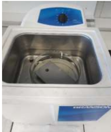
Figure 50: Ultrasonic bath apparatus containing a solution of 50% distilled water + 50% ethanol.
