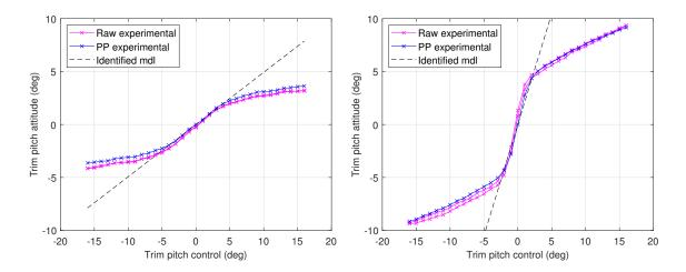
Figure 2.1 – Trim maps of the ACO projectile for different values of the geometric parameter:  $x_F = 0.313$  m (left) and  $x_F = 0.175$  m (right)
