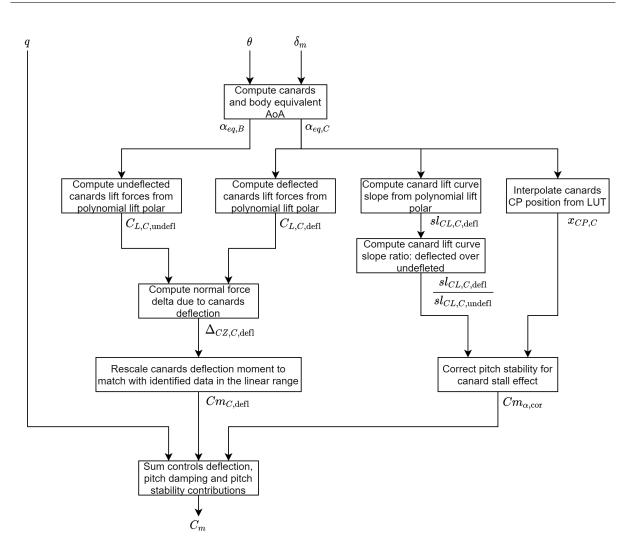
Figure 3.8 – Flowchart of the semi-local model
