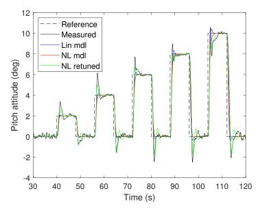
Figure 3.48 – Pitch attitude tracking of the RSS projectile
