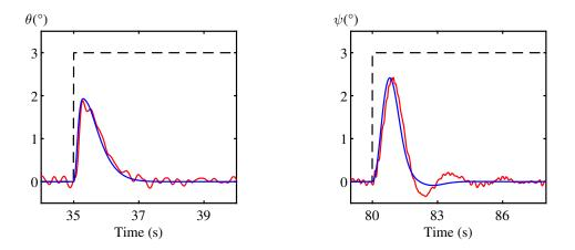
Figure 1.21 – Pitch (left) and yaw (right) disturbance rejection disturbance (dashed), simulation (blue) and measurements (red)
