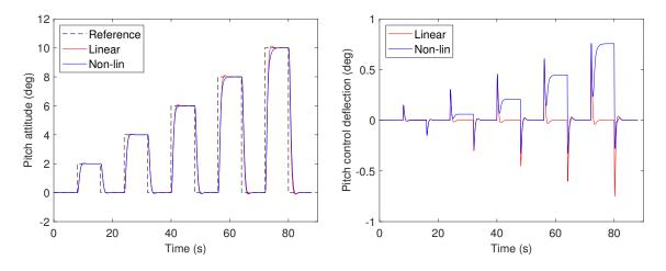
Figure 3.40 – Step tracking of the RSS projectile for increasing amplitudes
