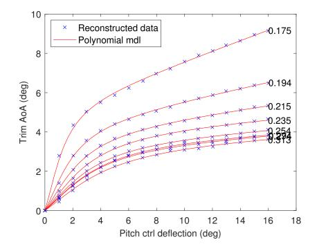
Figure 2.23 – Post-processed trim maps and polynomial models for different fins positions  $x_F$  (m)
