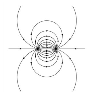
Figure 2.11 – Streamlines induced by a source-sink pair (reproduced from [HC03])
