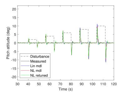
Figure 3.57 – Disturbance rejection of the dual-loop co-design
