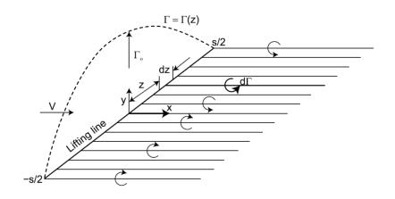
Figure 2.15 – Pradtl lifting-line model of the finite wing (reproduced from [HC03])
