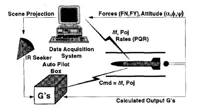
Figure 18 – The Virtual Flight Testing concept [RM95]
