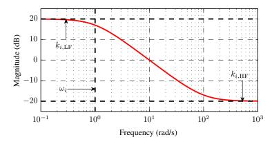
Figure 1.16 – Parametrization of the inverse filter  $W_i^{-1}$  [Str16]
