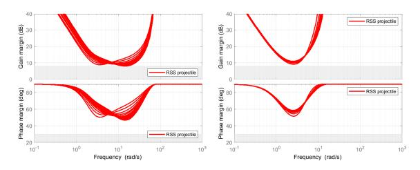
Figure 3.37 – Stability margins at the actuator input  $\delta_m$  (left) and at the output  $\theta$  (right)
