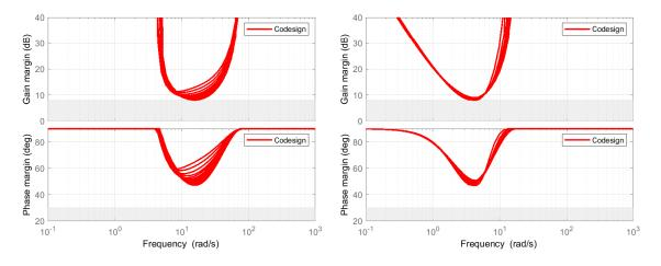
Figure 3.25 – Stability margins at the actuator input  $\delta_m$  (left) and at the output  $\theta$  (right)
