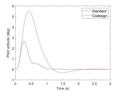
Figure 3.33 – Disturbance rejection of standard and optimized airframes
