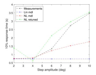
Figure 3.56 – Response time prediction and measurement
