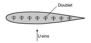
Figure 2.14 – Disposition of singularities for the lifting problem (reproduced from [HC03])
