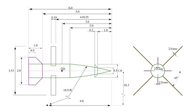
Figure 16 – Tri-surface gliding projectile concept [Olm16]
