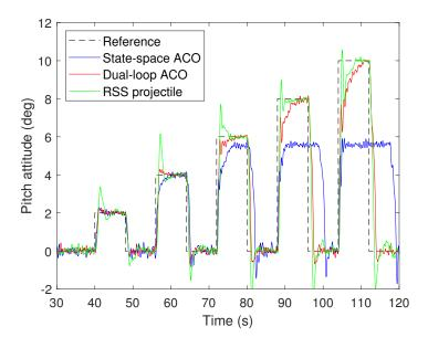
Figure 3.61 – Comparison of the measured step responses of the various agile projectile designs
