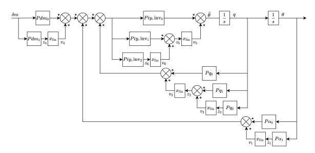
Figure 2.9 – Block diagram of the pitch dynamics model
