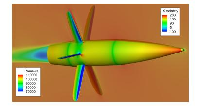
Figure 17 – CFD visualization of the pressure field around a projectile [Dec+18]
