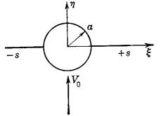
Figure 2.12 – Circular mid-wing airframe section into a uniform cross flow (reproduced from [Nie88])
