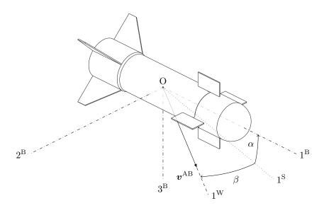
Figure 1.10 – Wind coordinate system [Str16]
