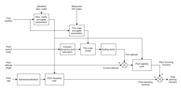
Figure 2.22 – FAST diagram of data-based model
