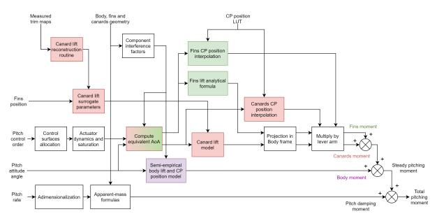
Figure 2.20 – FAST diagram of component-based model
