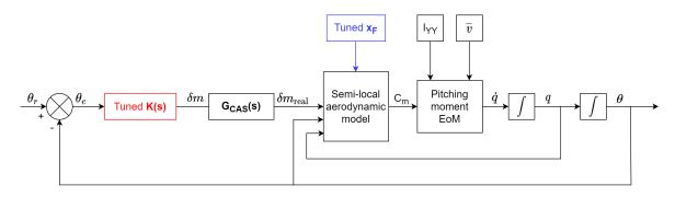
Figure 3.7 – Non-linear pitch dynamics simulator
