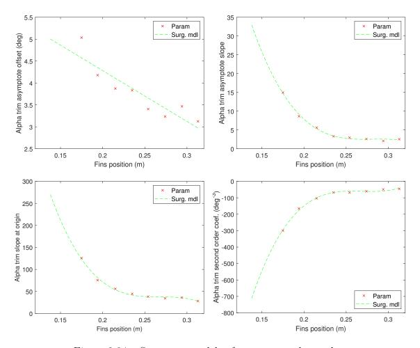
Figure 2.24 – Surrogate models of  $\alpha_{\text{aoff}}$ ,  $\alpha_{\text{aslp}}$ ,  $sl_{0,\alpha}$  and  $a_2$
