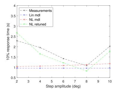
Figure 3.50 – Response time prediction and measurement
