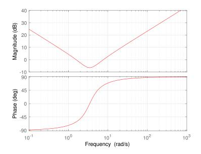
Figure 3.20 – Bode plot of the tuned dual-loop controller
