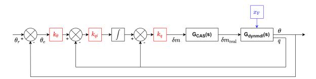
Figure 3.11 – Dual-loop controller structure
