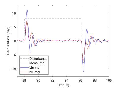
Figure 3.47 – Zoom on the 8° disturbance step rejection
