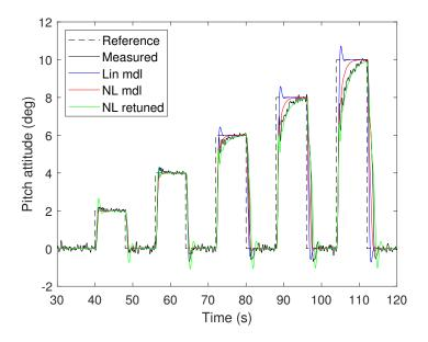
Figure 3.54 – Pitch attitude tracking of the dual-loop co-design
