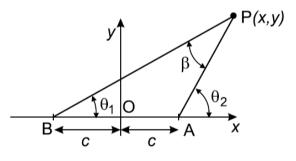
Figure 2.10 – Geometry of a source upstream of a sink (reproduced from [HC03])
