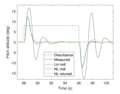
Figure 3.53 – Zoom on the  $8^\circ$  disturbance step rejection
