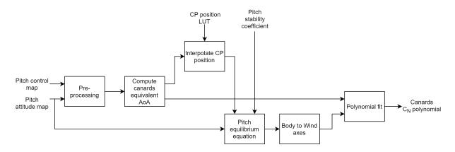
Figure 2.16 – FAST diagram of canard lift reconstruction routine
