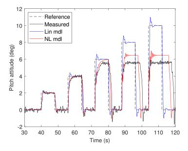
Figure 3.43 – Pitch attitude tracking of the state-space co-design
