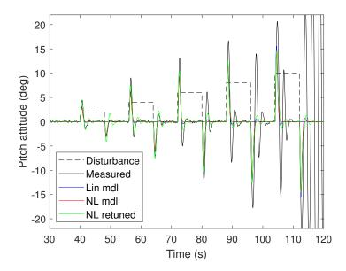
Figure 3.51 – Disturbance rejection of the RSS projectile
