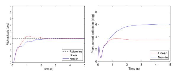
Figure 3.19 – Projectile step response at maximum control AoA
