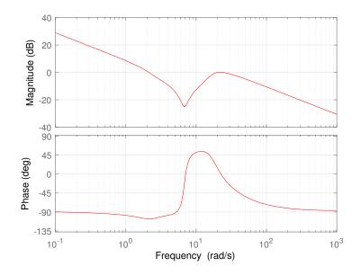
Figure 3.12 – Bode plot of the tuned state-space controller
