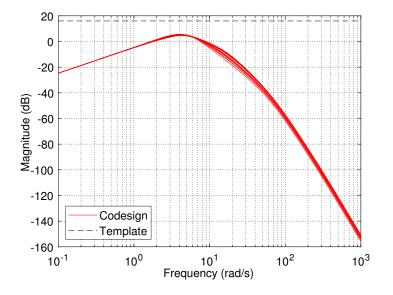
Figure 3.24 – Robustness transfer GS and associated template
