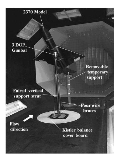
Figure 20 – The M2370 mock-up on its dynamic testing rig [GL06]
