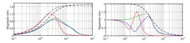
Figure 1.17 – Disturbance rejection transfers  $\mathbf{T}_{\mathbf{d}\to\mathbf{e}}$  (left) and  $\mathbf{T}_{\mathbf{d}\to\mathbf{u}_{\mathbf{c}}}$  (right) The roll (green), pitch (blue) and yaw (red) channels are compared to the templates (dashed for roll and pitch, dash-dotted for yaw); frequency is in rad/s
