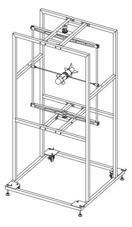
Figure 1.2 – 3 degrees-of-freedom gimbal assembly [Strub, 2016]
