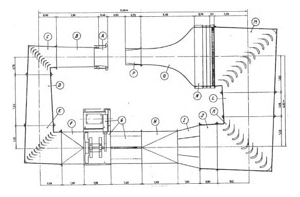
Figure 1.1 – ISL subsonic wind tunnel layout [Jaeggy, 1982]
