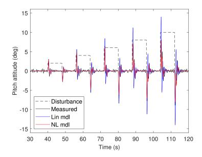
Figure 3.45 – Disturbance rejection of the state-space co-design
