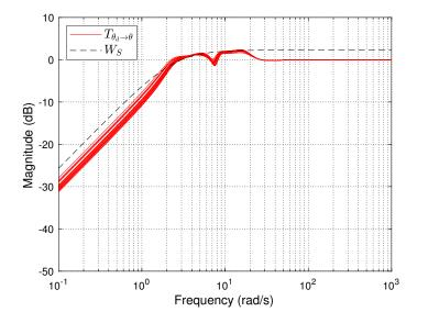
Figure 3.14 – Disturbance rejection transfer S and associated template
