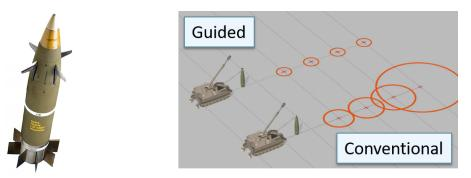
Figure 11 – The Excalibur projectile (left) and its range-independent dispersion (right)
