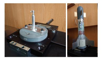
Figure 1.12 – CG position measurement setup for transverse (left) and base (right) planes
