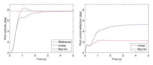
Figure 3.27 – Projectile step response at maximum control AoA
