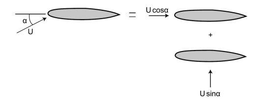
Figure 2.13 – Principle of superposition: lifting (bottom) and non-lifting (top) problems (reproduced from [HC03])
