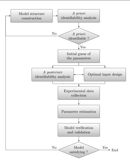
Figure 1.11 – System identification procedure [Str16]
