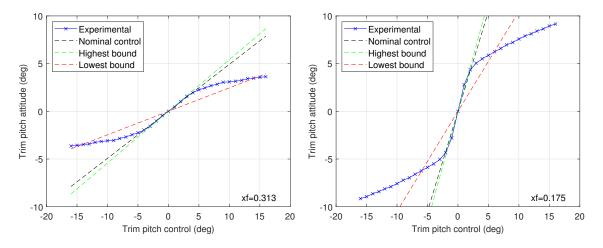
Figure 3.5 – Comparison of uncertain pitch control model with measured trim maps for different fins positions
