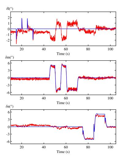
Figure 1.20 – Actuator deflection during tracking simulation (blue) and measurements (red)
