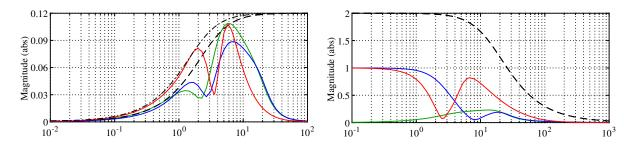
Figure 1.18 – Reference tracking transfers  $\mathbf{T}_{\mathbf{r}\to\mathbf{e_{mm}}}$  (left) and  $\mathbf{T}_{\mathbf{r}\to\mathbf{u_c}}$  (right) same legend as above
