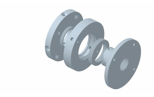
Figure 1.3 - CAD of the redesigned roll sleeve
