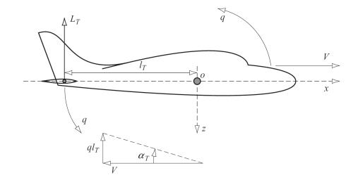
Figure 2.6 – Tailplane incidence due to pitch rate [Coo12]
