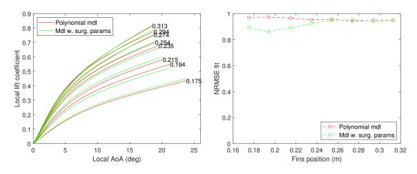
Figure 2.19 – Canard lift polars for specified  $x_F$  (left) and models fit (right)
