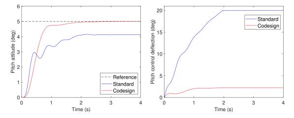
Figure 3.32 – Reference tracking of standard and optimized airframes
