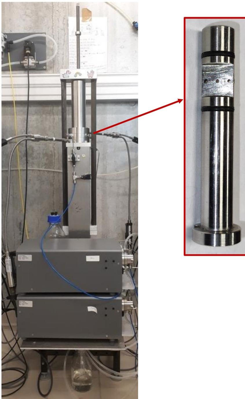
Figure 4.2. Pictures of the continuous pneumatic elongational-flow reactor and mixer (cpRMX, left) and the mixing element (right).
