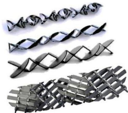
Figure 1.35. Different static mixers designs [219].
