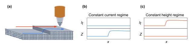
Figure 1.4: **Different scanning regimes.** (a) Sketch of the junction of the scanning tunneling microscope. Blue line represents the constant current regime and the red line represents the constant height regime. (b) Scanning in a constant current regime. (c) Scanning in a constant height regime.
