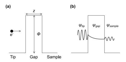
Figure 1.2: Quantum tunneling phenomena. (a) Sketch of the potential barrier at the classical limit. The potential barrier of height  $\Phi$  is created by the gap between two electrodes. The electron  $e^-$  with energy  $E < \Phi$  is travelling from the tip on the left to the sample on the right but is bounced back (reflected) at the barrier. (b) Sketch of the quantum mechanics interpretation where the electron is pictured as a wave.
