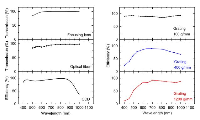
Figure 1.8: Transmission and efficiency of the optical elements. Left: transmission percentage for the AC254-050-B focusing lens and optical fiber SEDI ATI 4x200  $\mu m$  and efficiency of the CCD. Right: efficiency of the three gratings of the spectrometer.
