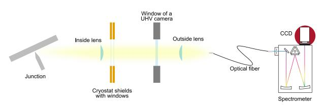
Figure 1.7: Sketch of an implemented light collection system. The light emitted at the tip-sample junction is collected by a first lens and directed outside of the vacuum chamber to be collected by the outside lens and coupled into optical fiber. The light is then guided by fiber into the spectrometer. The sketch of the spectrometer is obtained from the Princeton Instruments manual.
