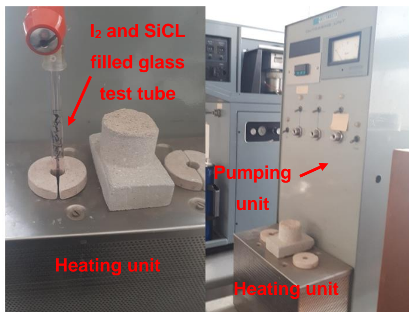
Figure 3.3 Adapted BET heating and pumping unit used for the iodine annealing of the silicon clathrates films.
