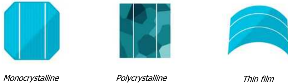
Figure 1.5.: The main types of the PV cell [1].
