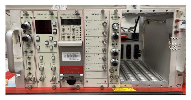
Figure 22. Alpha spectrometer used to measure the detector resolution.
