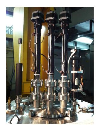
**Figure 14.** Three telescoping arms attached to the ladders allowing the remote control over them. Reprinted from ref. [113].
