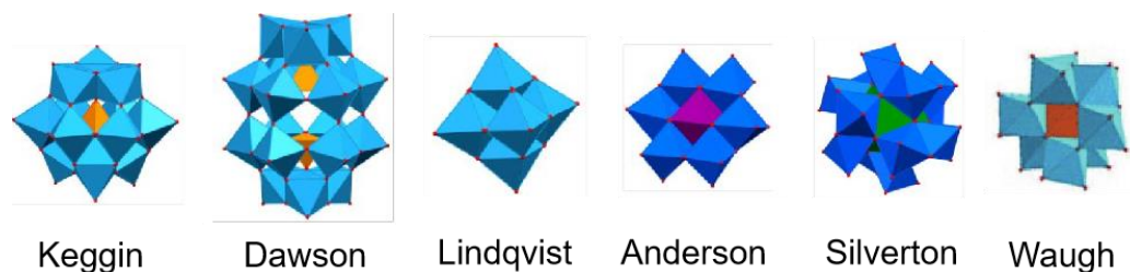
Figure 1.1.1 Six typical structures of polyoxometalates: Keggin, Wells-Dawson, Lindqvist, Anderson-Evans, Silverton, and Waugh.
