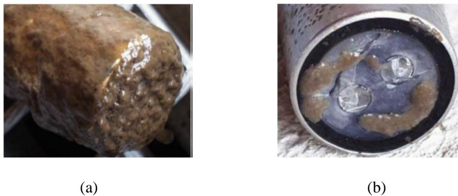
Figure 7.21 Biofouling effect in optical turbidimeter: (a) after 30 days in a wastewater treatment plant, (b) after ultrasonic cleaning.
