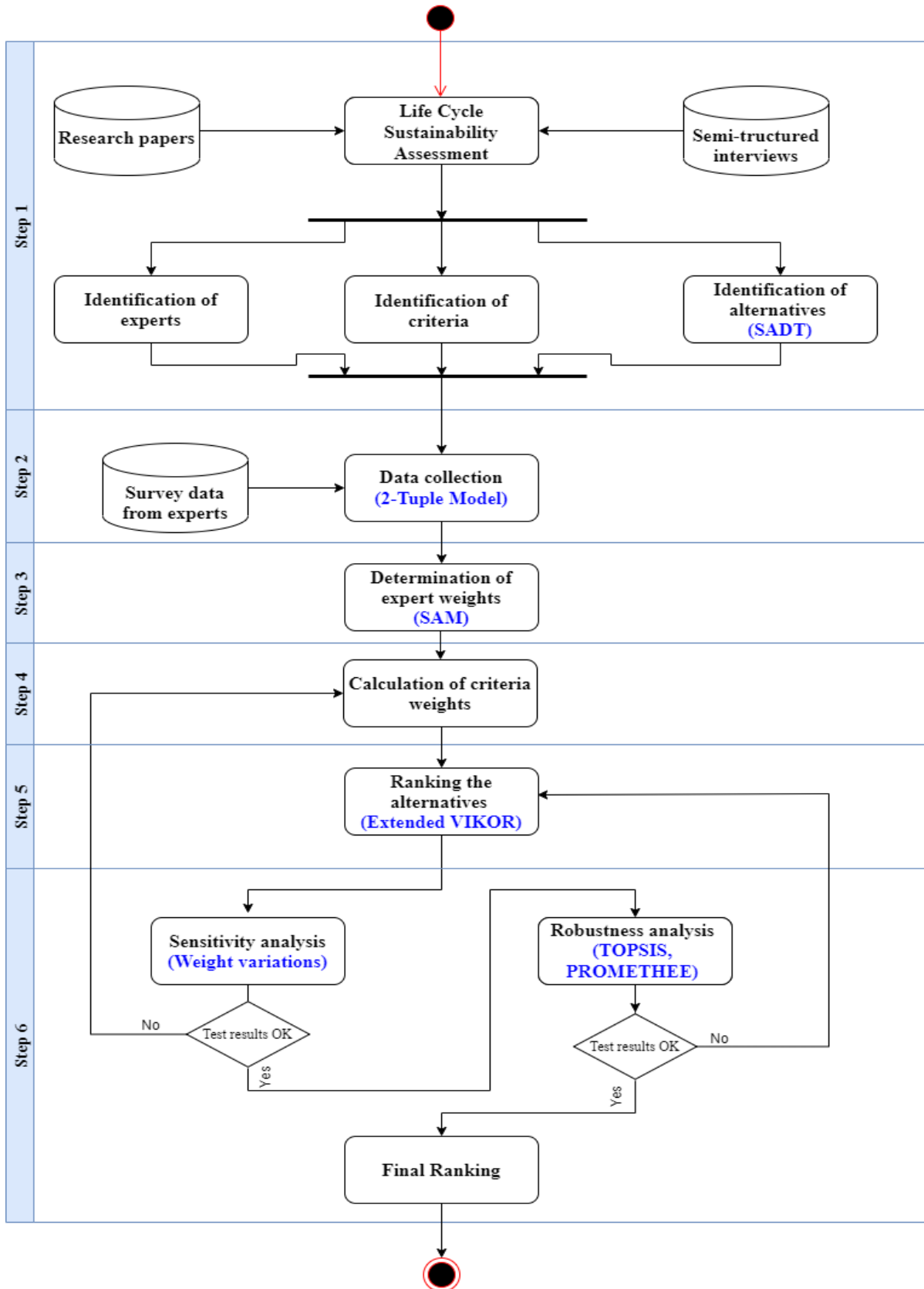
Figure 30: Process diagram of the proposed framework
