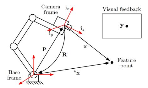
Figure 4.1: Diagram representing the typical set-up of the visual-servoing method. Image adapted from [Navarro-Alarcon and Liu, 2014]
