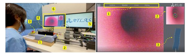
Figure 4.8: Multi-level-assistance robotic platform. a) The general perspective of the platform. b) The User Interface. Image adapted from [Finocchiaro et al., 2022].
