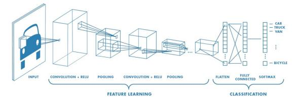
Figure 2.2: Typical architecture of a CNN. Image adapted from [MathWorks, 2017]
