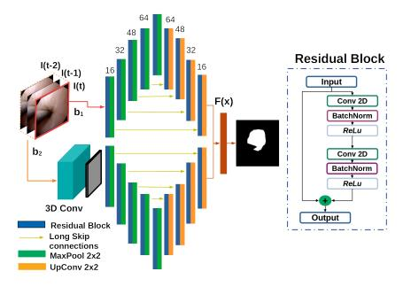
Figure 4.3: Architecture used for lumen segmentation. The CNN is composed of two branches, both of which are composed of residual blocks. Branch  $b_1$  process the information of the current frame, while  $b_2$  considers the information of the current, and three previous frames I(t). The final output combines the predictions of both branches in the last layer using the ensemble function F(x)
