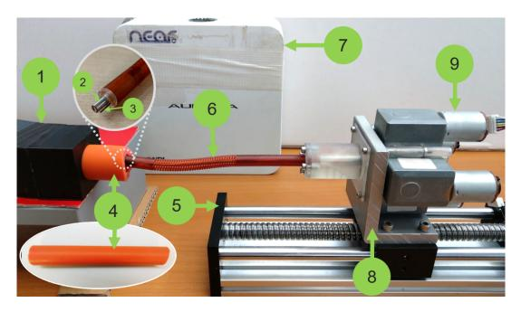
Figure 4.2: Assembly of the actuation platform for the soft robotic endoscope and the experimental set-up for the system validation: 1) 3D printed mold to fix the curve of the lumen phantom; 2) Endoscopic camera; 3) Electromagnetic tracking sensors on the robot tip: 4) Soft anatomical phantom; 5) Linear stage; 6) Soft robotic arm 7) Electromagnetic field generator; 8) Linear actuation module; 9) DC motors
