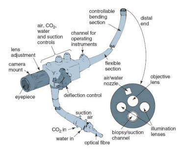
Figure 1.3: Diagram of a current endoscope. Image adapted from [Graeme, 2003]
