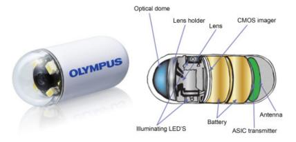
Figure 1.9: Small intestine capsule endoscope. Image adapted from [Olympus, 2013].
