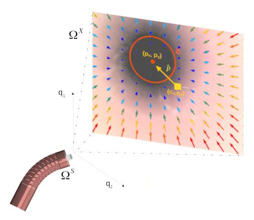
Figure 4.5: Diagram depicting the main idea of the Artificial Potential Well approach. The robot tries to adjust its configuration  $\Omega^S$  by actuating  $q_1$  and  $q_2$ , to match the the center of the image plane  $(c_x, c_y)$  to the detected center of the lumen  $(p_x, p_y)$  An overlay view from the endoscopic camera and the 2D representation of the potential well is depicted on the right.
