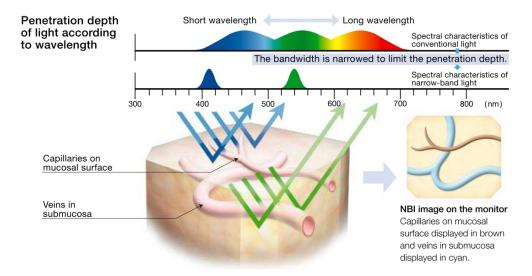
Figure 3.1: Working principle of Narrow Band Imagining. Image adapted from: [Lukes et al., 2013]
