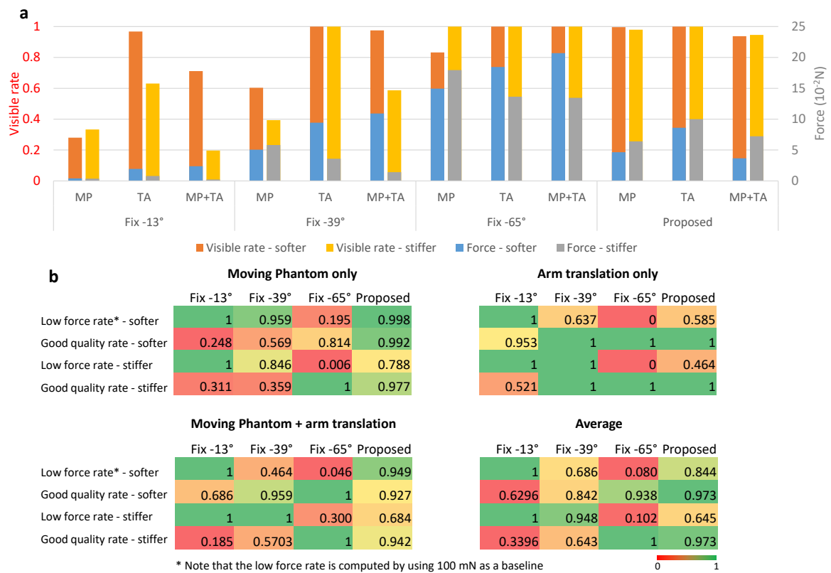
Fig. 4.13 Force vs scanning quality on phantoms with two levels of stiffness. (a) visualizes The average force and visible rate, under conditions of moving phantom only (MP), translating arm only (TA) and a combination of these two motions (MP + TA). (b) Shows the heat map of low force rate and good imaging quality rate.
