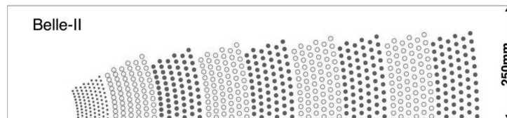
Figure 2.9: Layout of the CDC 9 wire superlayers. The innermost superlayer is made of two layers while the other are composed of six layers each. Image from [77].
