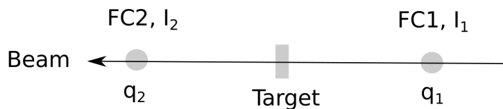
Figure 2.18: Scheme of the Faraday cups system used in the STELLA experiment before and after the target, measuring intensities I_1 , I_2 at charged states q_1 , q_2 [40].
