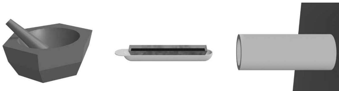
Figure II.1. Scheme of the tools used for the ceramic method. From left to right: agate stone mortar, alumina basket with platinum foil and tubular furnace.
