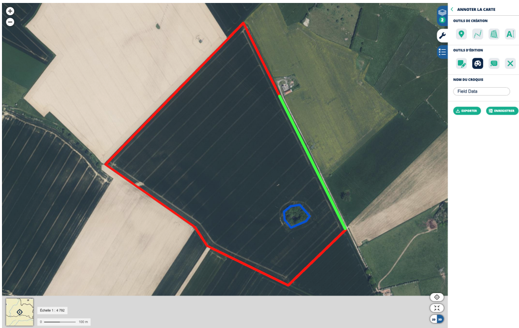
FIGURE 3.1: The Géoportail [45] annotation tool. a field polygon, an obstacle inside it and one access segment are annotated in red, blue and green
