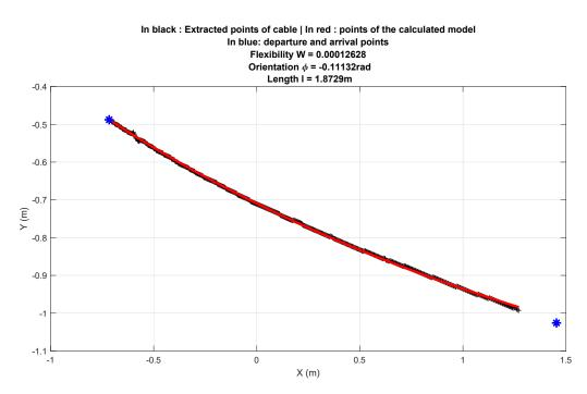
Figure 3.12: The validation of the geometric model of flexible cable from the video stream.
