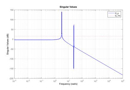
Figure 4.7: Frequency behavior of the open-loop nominal system
