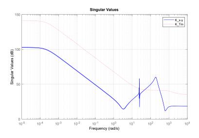
Figure 4.8: Frequency behavior of the controller
