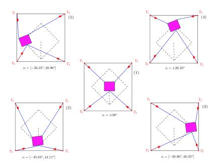
Figure 2.14: The platform's possible orientation in different locations in the workspace.
