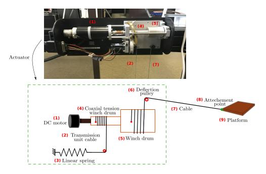
Figure 2.3: Actuator scheme of the INCA robot prototype.
