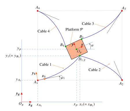
Figure 3.2: Schematic representation of a planar four flexible cable robot.
