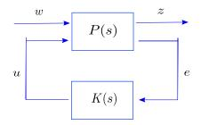
Figure 4.2: Standard scheme of the  $\mathcal{H}_{\infty}$  synthesis
