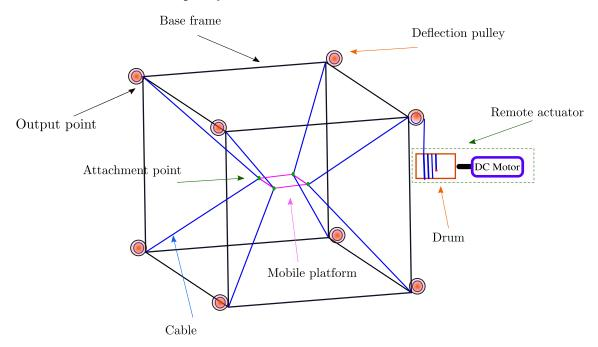
Figure 1.3: Elements of cable-driven parallel robot.
