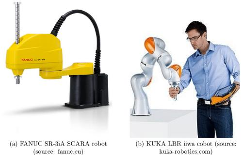
Figure 1.1: Serial robots (Cobot and SCARA robot)
