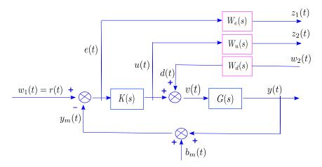
Figure 4.4: Four-block standard  $\mathcal{H}_{\infty}$  synthesis scheme with weighting functions
