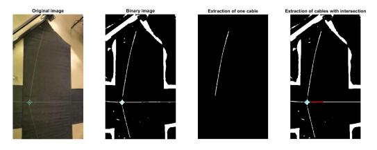
Figure 3.9: Extraction of cable from stream video (a. original image b. binary image c. extraction of one cable d. extraction of cables with intersection).
