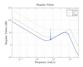
Figure 4.20: Frequency response of the controller
