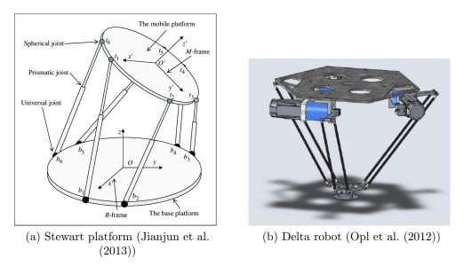
Figure 1.2: Parallel robots (Stewart platform and Delta robot)
