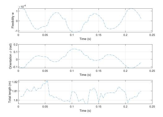
Figure 3.13: The time evolution of the estimated cable's variables  $(l,\varphi,w)$
