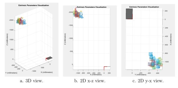
Figure 3.11: 3D representation of the position of our mobile camera in relation to the different views of the fixed calibration pattern.
