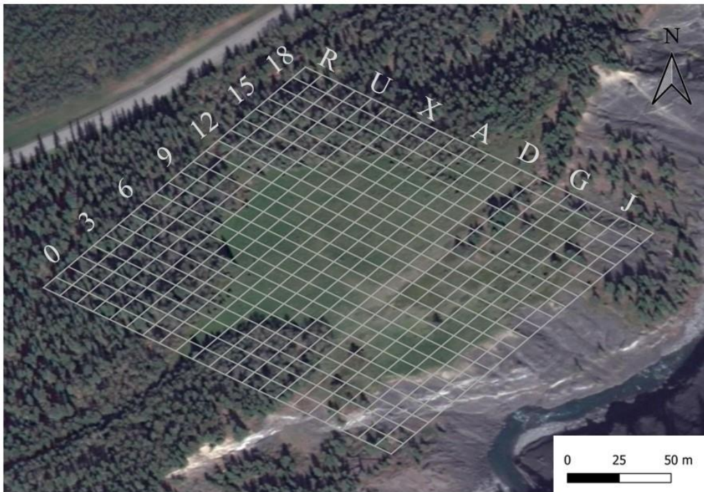
Figure 16. Example of the Cartesian grid on MB, lines every 10 m and resolution \pm 1 m.
