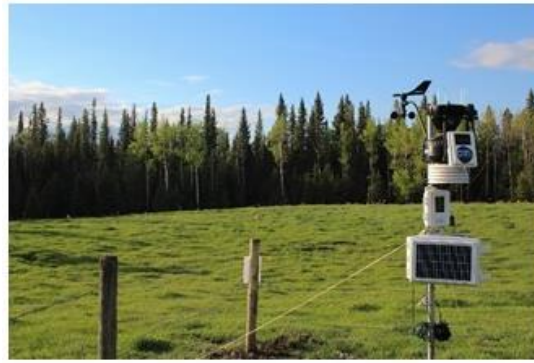
Figure 23. Example of the weather station on MB (on a nice day!) with the temperature sensor in the white shaded and ventilated area, the anemometer, and the rain collector (Davis, Vantage Pro2).
