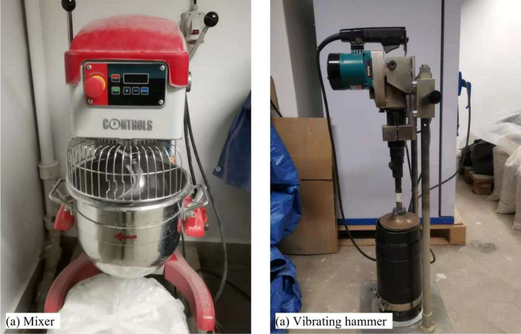
Figure II.9. Sample preparation equipment: (a) Mixer; (b) Vibrating hammer
