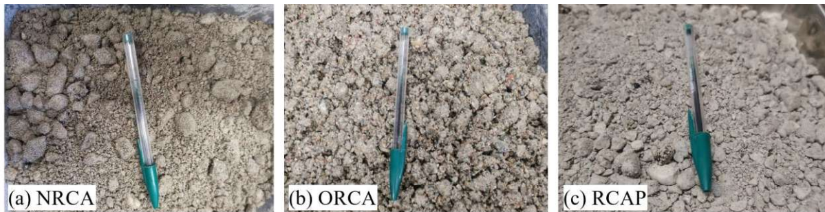
Figure II.1. Studied RCA materials: (a) NRCA; (b) ORCA; (c) RCAP
