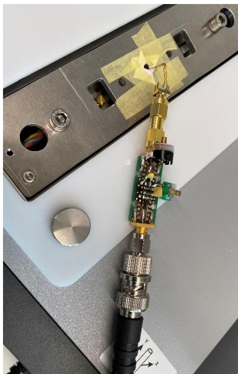
Figure 89 - Self-made miniaturized NMR receiving coil and its impedance matching board.
