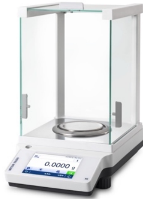
Figure 28: Analytical balance used to record the solvent evaporation rate.
