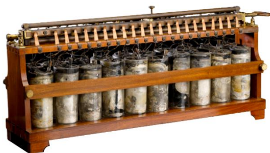
Figure 12: Initially designed lead-acid battery by Gaston Planté in the early 1860's (left) 62 ; Charge-discharge mechanisms of a lead-acid battery
