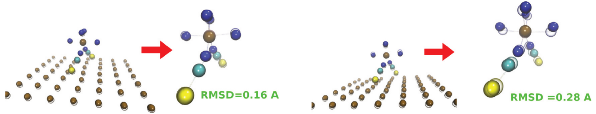
FIGURE 2.2 – Superposition on the iron atom of the octahedral and (NCS) groups of the relaxed H-Fephen and F-Fephen molecules on the substrate in the two magnetic state (LS-left, HS-right), in color for the F-Fephen, and transparent for the H-Fephen. Reproduced from [173].
