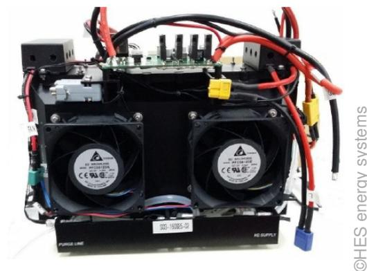
Figure 1.20: PaC Aerostak 1000 W
