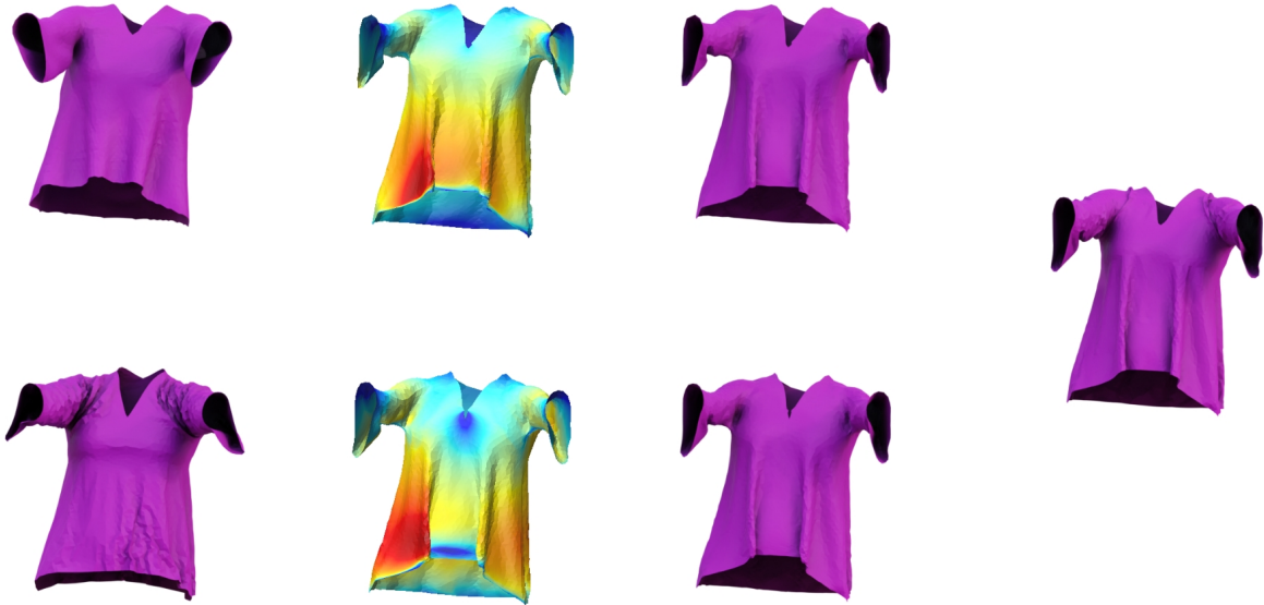
Figure 4.7: Robustness to different source meshes: the leftmost column displays the source meshes (with the upper images posed by LBS and the lower images draped by simulation), the second column shows the qualitative colormap of displacement magnitude, the third column presents the deformed meshes, and the rightmost column depicts the target mesh.
