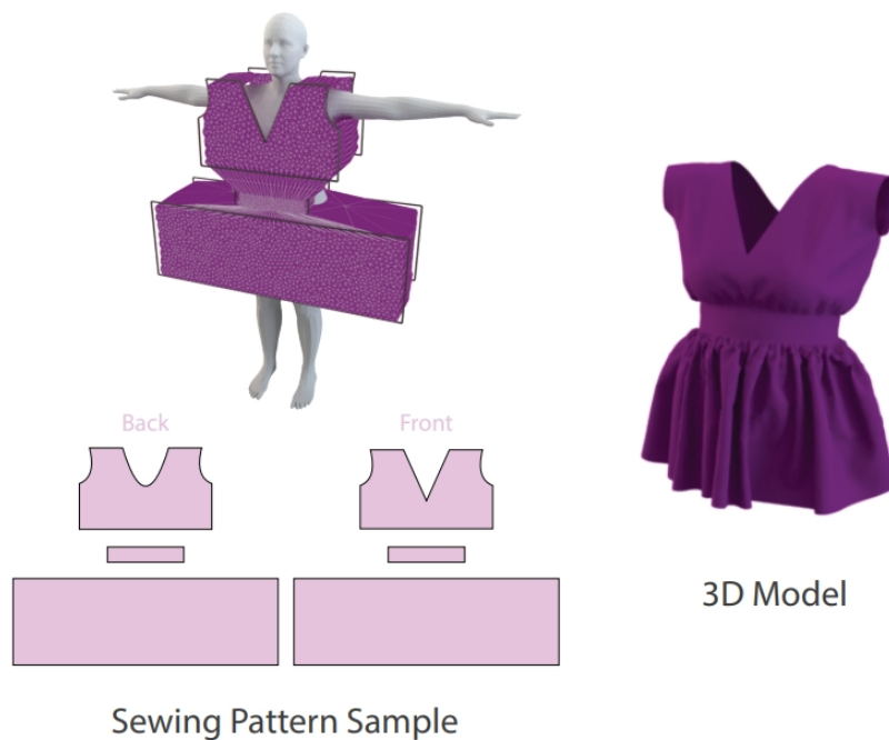
Figure 1.2: Sewing pattern samples are placed and draped over a body to get the corresponding 3D garment model, drawn from Korosteleva et Lee (2021) .
