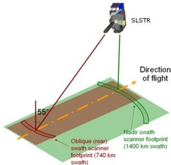
Fig 2.2 Track and scanning parameters of the Sentinel-3 SLSTR instrument with the nadir and oblique view (Credits: European Satellite Agency).
