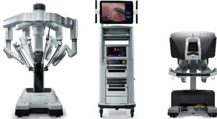
Figure 3.4: Components of the da Vinci Surgical System: Patient Side Cart, Vision Side Cart, and Surgeon Console. (Image courtesy of [Avgousti 2020])
