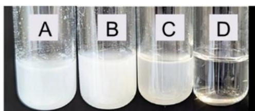
Figure 18: Preparation of pegylated phosphines. (a) Synthesis of water-soluble pegylated phosphines. (b) Solubility of different triphenylphosphines in water (3 mg/mL).
