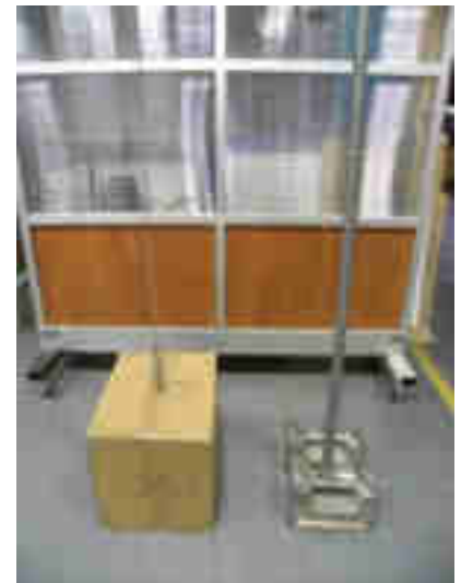
Figure 39 : Essai impact concentré [78]
